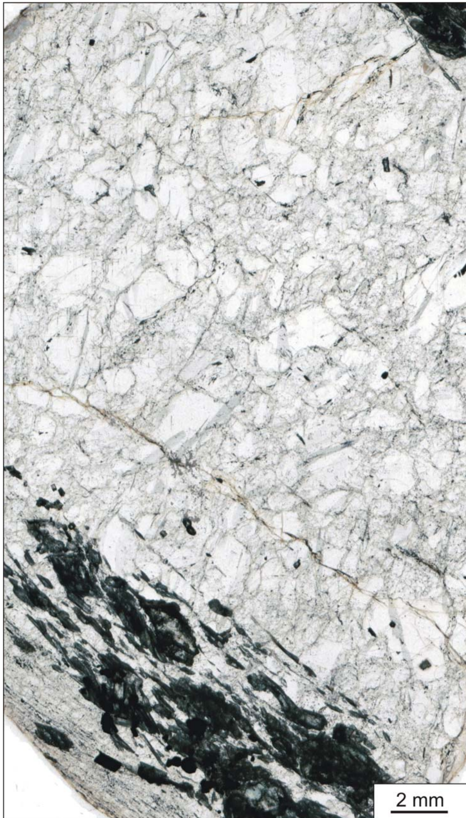
Figure 32. 500 \mu\text{m} -thin section scan of a quartz layer in the Nasafjell kyanite quartzite. Black – kyanite, white – quartz.
