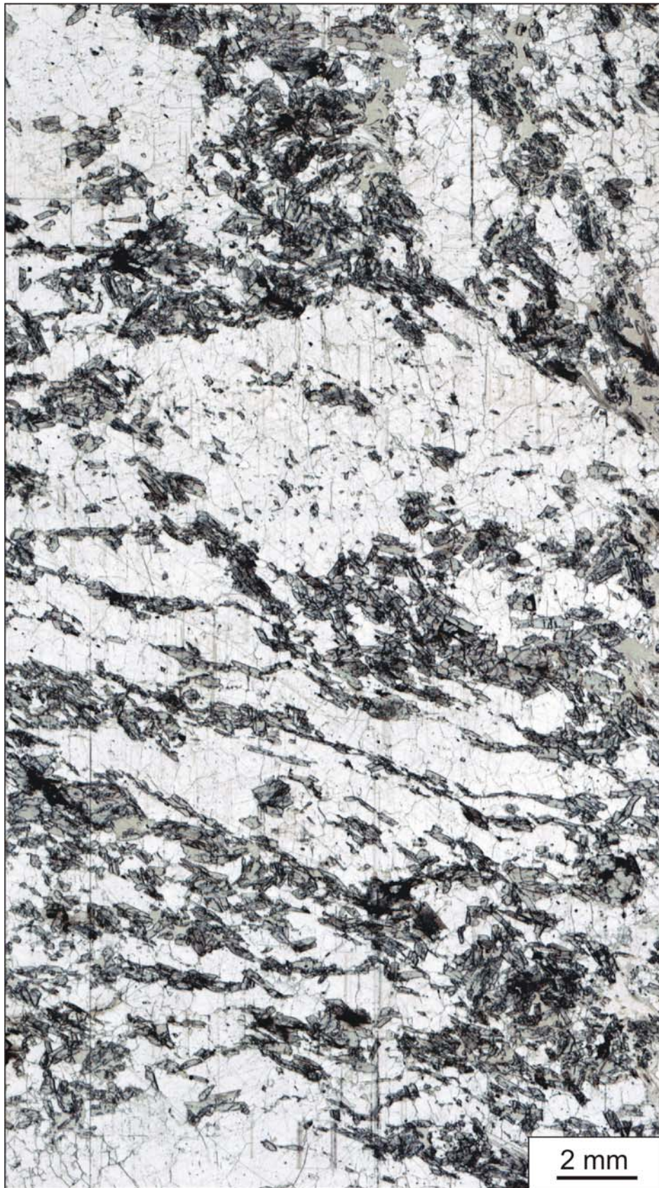
Figure 22. Thin section scan of a kyanite-rich layer in the Gullsteinberget kyanite quartzite. Dark grey – kyanite, bright grey – pyrophyllite/muscovite, white – quartz.
