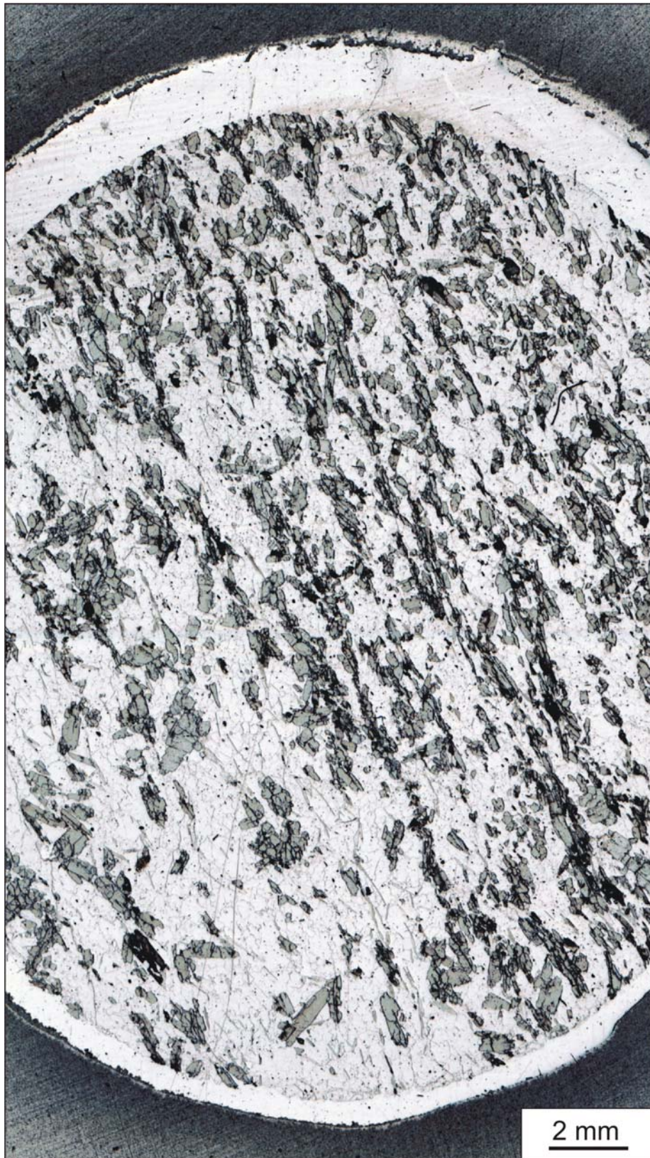
Figure 29. Thin section scan of a kyanite-rich layer in the Tverrådalen kyanite quartzite (drill core). Dark grey – kyanite, black – sericitised kyanite, white – quartz.
