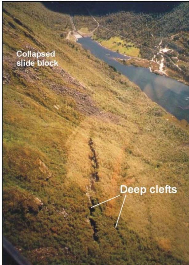
**Figure 42.** Open fractures further west. The cleft is situated in a collapsed part of the mountain slope (see locality in Fig. 38). View is to the SE.
