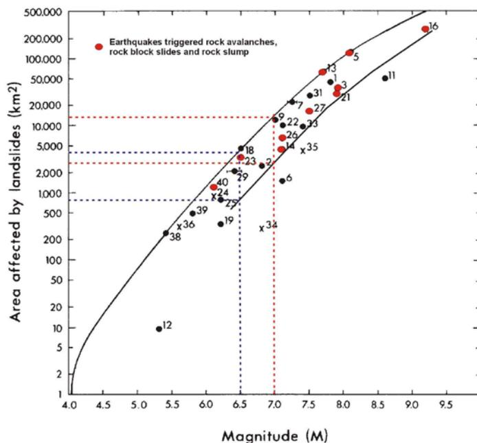
**Figure 48.** Area affected by landslides in earthquakes of different magnitudes (after Keefer, 1984). Events triggering rock avalanches, rock-block slides, and rock slumps, are shown in red. Areas affected by landslides during earthquakes of 6.5 and 7.0 are indicated. An earthquake of M 6.5 would for example imply an area affected by landslides of between 800 and 4000 km<sup>2</sup>.
