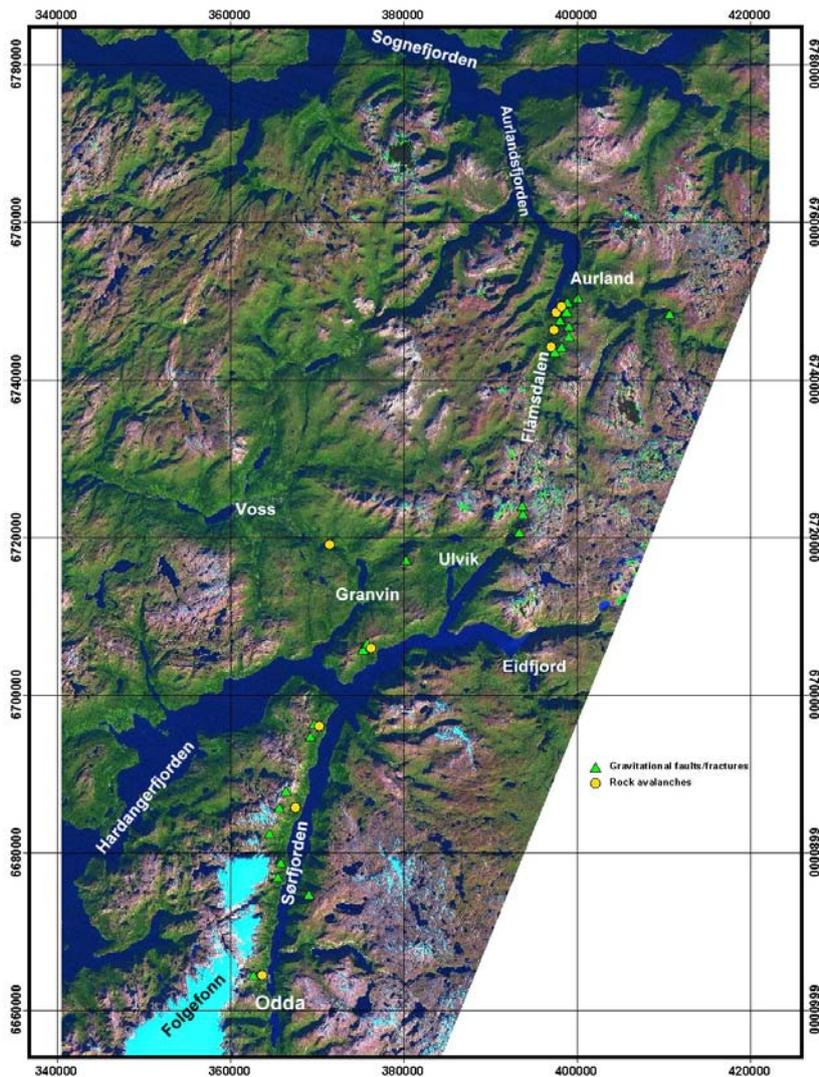
**Figure 45.** Satellite image showing locations of gravitational-slope failures in an area from Odda in Hardanger to Aurland in Sogn. An interpretation of aerial photographs has been conducted in a 20 km wide area from Odda to Aurland. The line spacing is 20 km. From Blikra *et al.* (2000A).
