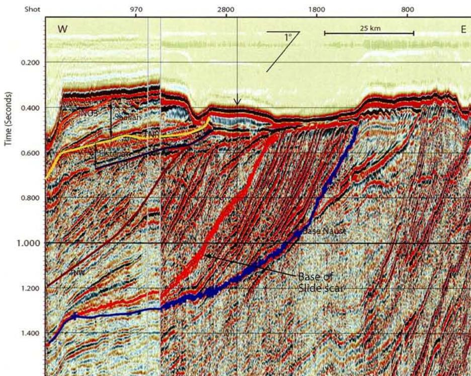
Figure 8.4.1A Seismic line MB 15-84 across a possible paleo-slide scar. The scar is approximately 25-30 km wide and 200 ms deep. The arrow marks the intersection between profiles 14 and 15. See figure 8.1 for location.
