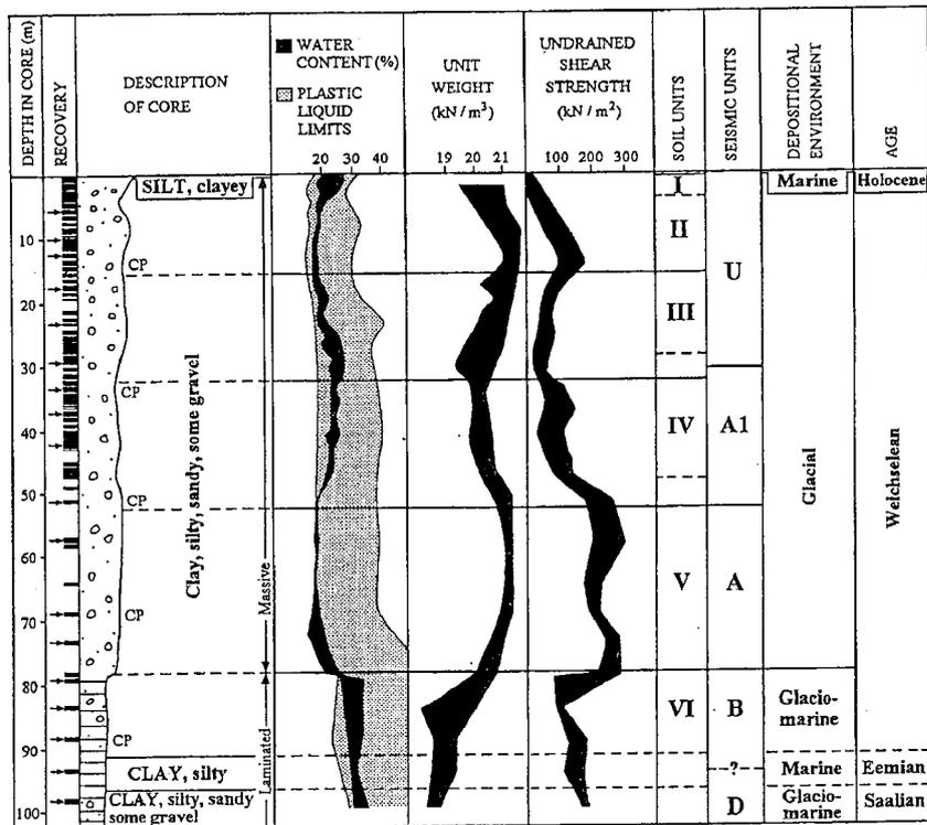
Figure 7.2.1 Summary of geotechnical boreholes in the Smørbukk South Platform area. Seismic units IKU-U, -A1 and A represent Weichselian deposits. Eemian sediments are found within unit IKU-B, corresponding to horizon INO3 in the present report (after Sættem et al. 1996).
