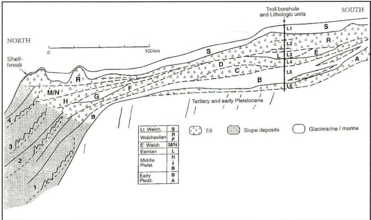
Figure 3.3.3 Profile along the Norwegian Channel from south of borehole 8903 and towards the North Sea Fan (after Sejrup et al. 2000).
