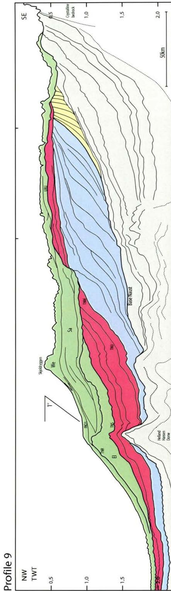
Figure 5.2.10 Line drawing of seismic composite profile 9 across Sklinnabanken and northern part of Haltenbanken to the shelf edge, across Skjoldryggen and down the slope onto the Vøring Plateau. Yellow – Oligocene deltaic unit. Blue – Naust W, red – Naust U & S, green – Naust R & O. We = Weichselian, Sa = Saalian, El = Elsterian. See figure 5.2.1 for location and table 5.2.1 for reference to applied seismic lines.
