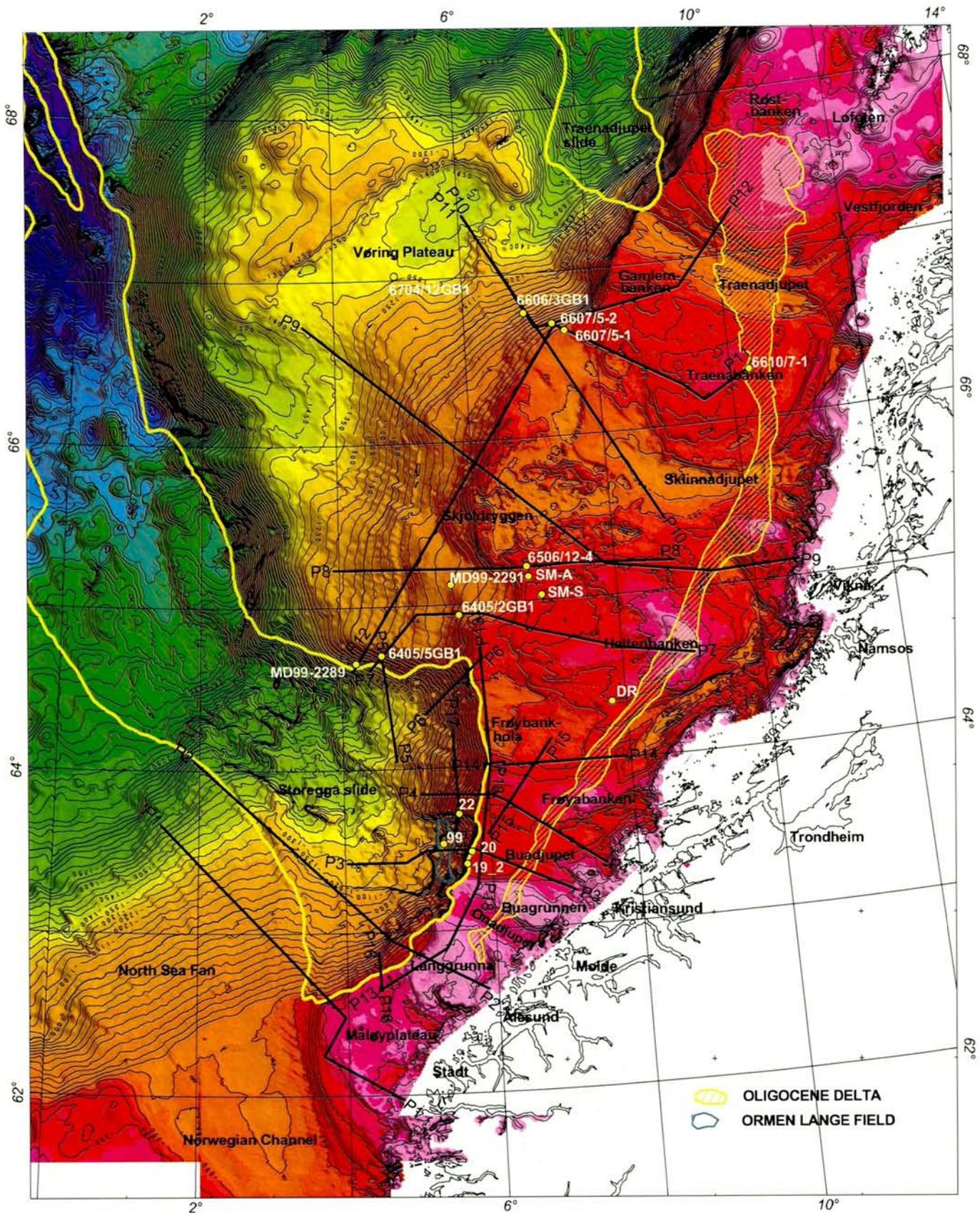
Figure 5.2.1 Bathymetric map with presented seismic profiles, exploration wells and geotechnical drilling sites. The profiles are either presented as data examples and/or line drawings. See table 5.2.1. DR-Draugen, SM-S – Smørbukk South, SM-A – Smørbukk Alfa.
