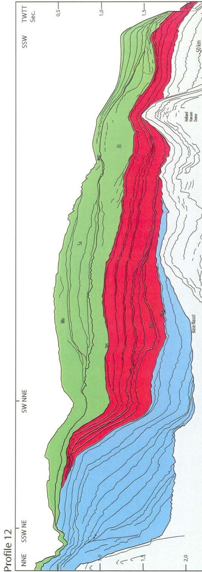
Figure 5.2.15 Line drawing of seismic composite profile 12 from the northern part of the Storegga slide across the outer shelf (Skjoldryggen) north-west of Haltenbanken and onto outer Trænabanken area, across Trænadjupet to Røstbanken. Blue – Naust W, red – Naust U & S, green – Naust R & O. We = Weichselian, Sa = Saalian, El = Elsterian. See figure 5.2.1 for location and table 5.2.1 for reference to applied seismic lines.
