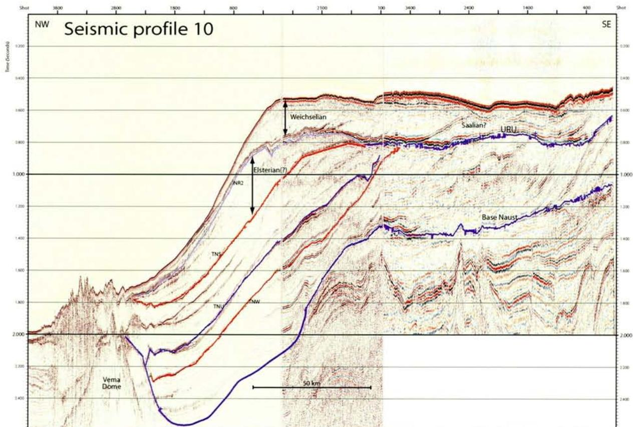
Figure 5.2.13 Interpreted seismic composite profile 10. Note that the angular unconformity (URU) is well defined, and that URU seems to be related to the deposition of unit R3 (Elsterian?). The Saalian Ice Sheet did not extend to the shelf edge west of Trænabanken. See figure 5.2.1 for location and table 5.2.1 for reference to applied seismic lines.
