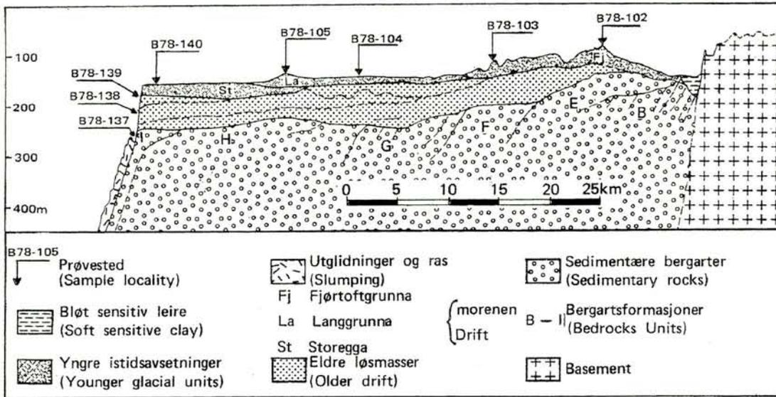
Figure 3.3.5 SE-NW profile showing interpreted bedrock units and Quaternary sediments at c. 63°N (Langgrunna) (after Rokoengen 1980).
