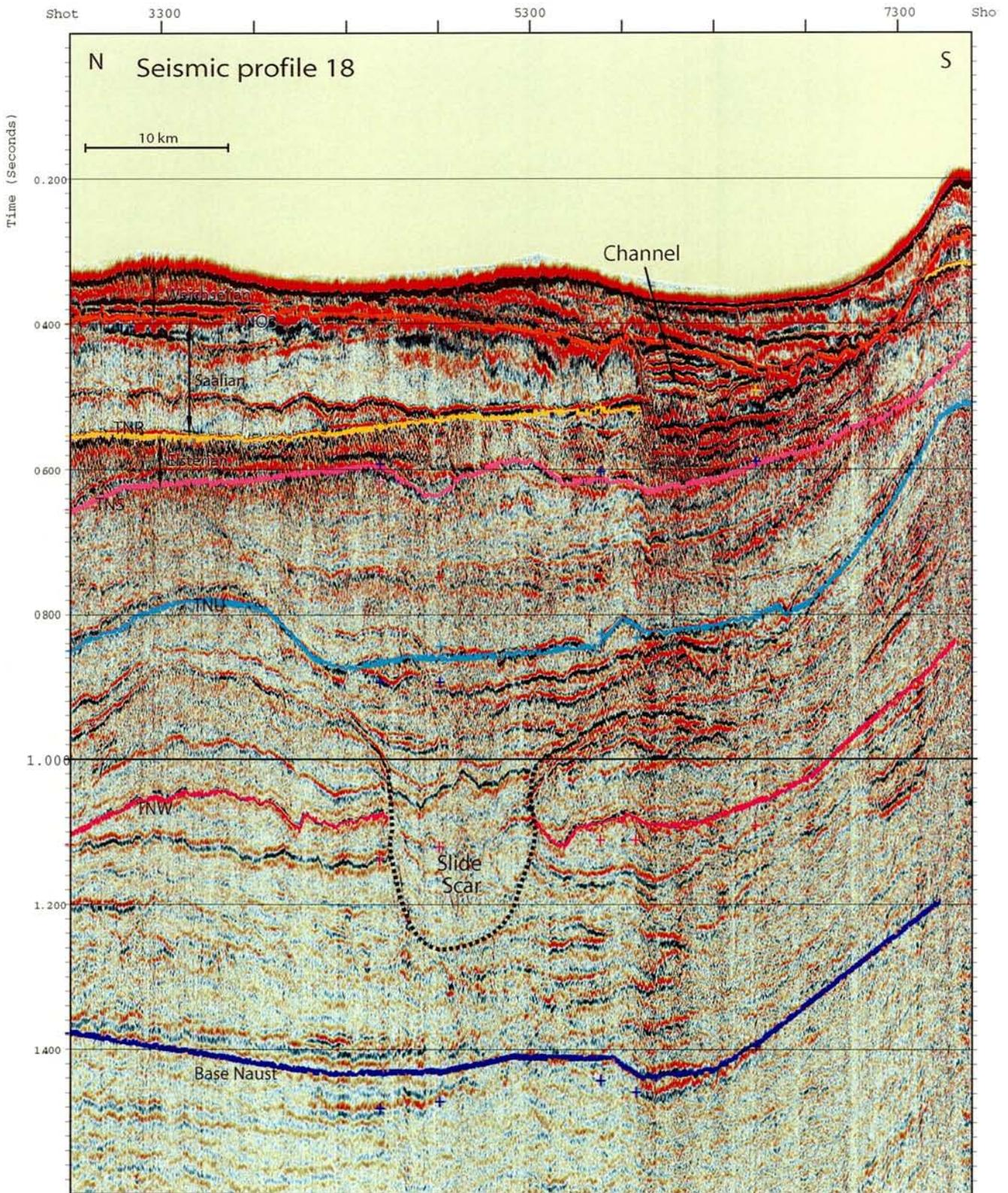
Figure 8.1.1 Seismic line NH0163-1303 along the outer shelf between Buagrunden and Frøyabanken west (northern end). Note the infilled subglacial channel of Late Saalian age and the slide scar near the TNW horizon. The line segment is a part of profile 13 (Fig. 5.2.17B). See figure 8.1 for location.
