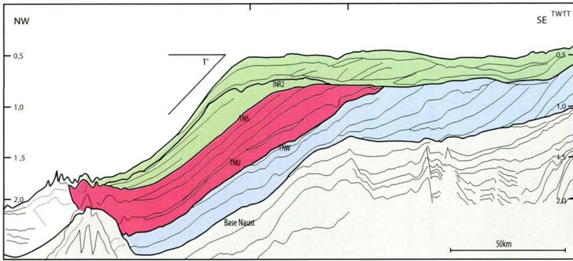
Figure 5.2.12 Line drawing of seismic composite profile 10 along outer Sklinnadjupet to the shelf edge and down the slope to the Vema Dome on the inner Vøring Plateau. Blue – Naust W, red – Naust U & S, green – Naust R & O. See figure 5.2.1 for location and table 5.2.1 for reference to applied seismic lines.
