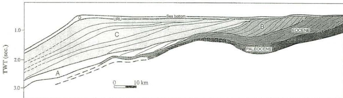
Figure 3.2.3 Schematic cross section of the Cenozoic stratigraphy on the northern part of the mid-Norwegian continental shelf. Unit C represents the Late Pliocene/Pleistocene prograding sequence (after Henriksen and Vorren 1996).
