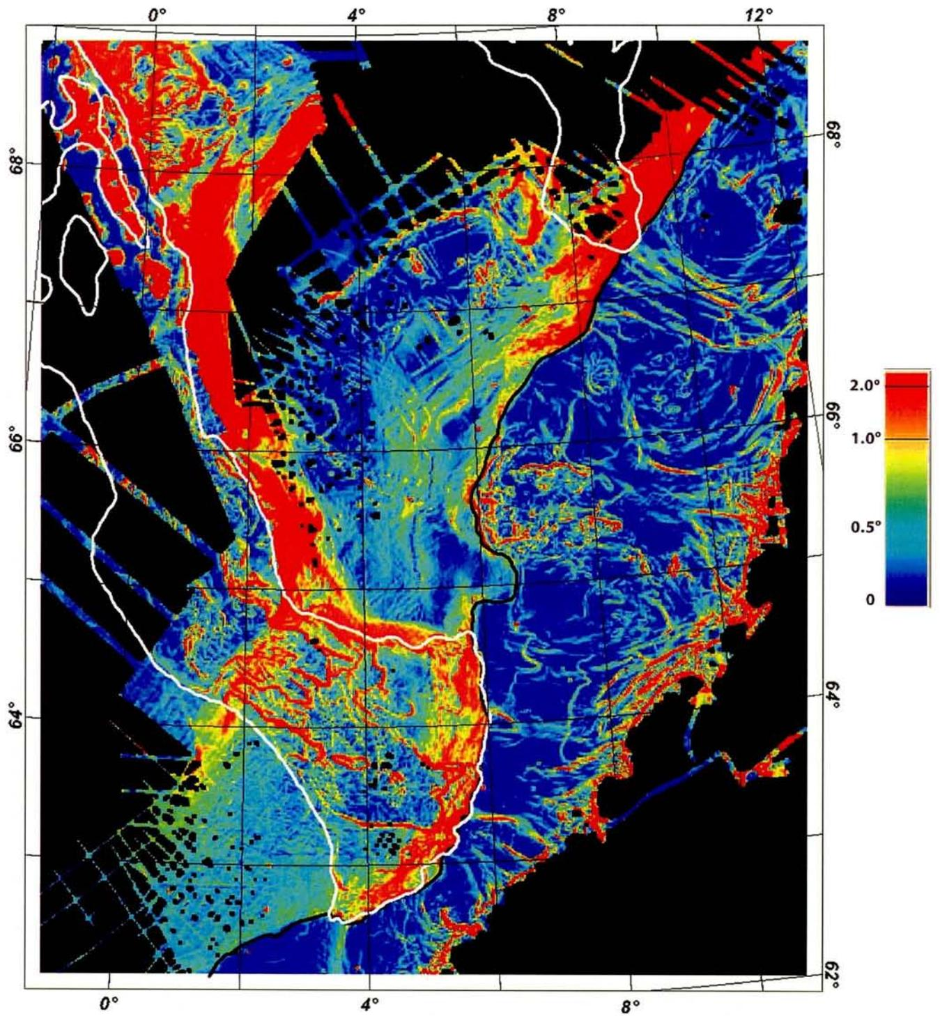
Figure 8.2 Slope inclination map of the mid-Norwegian margin.
