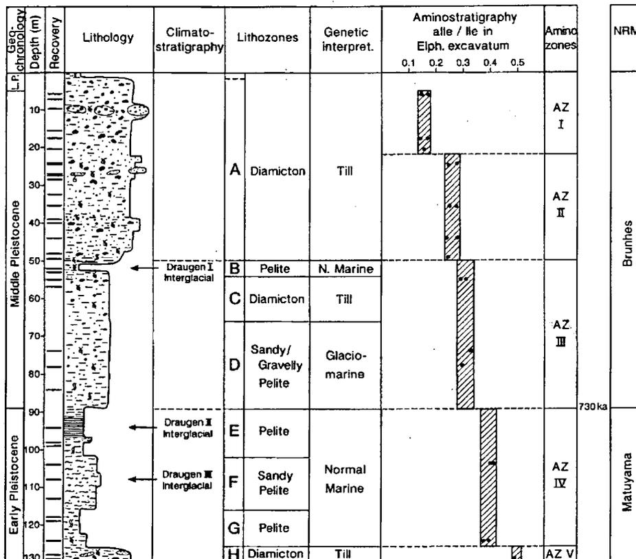
Figure 7.2.2 Genetic and chronostratigraphical interpretation of a geotechnical core at the Draugen platform site (after Hafliðason et al. 1991). Lithozones B to H corresponds to unit IKU-I, which in this study is a part of Sequence Naust W.
