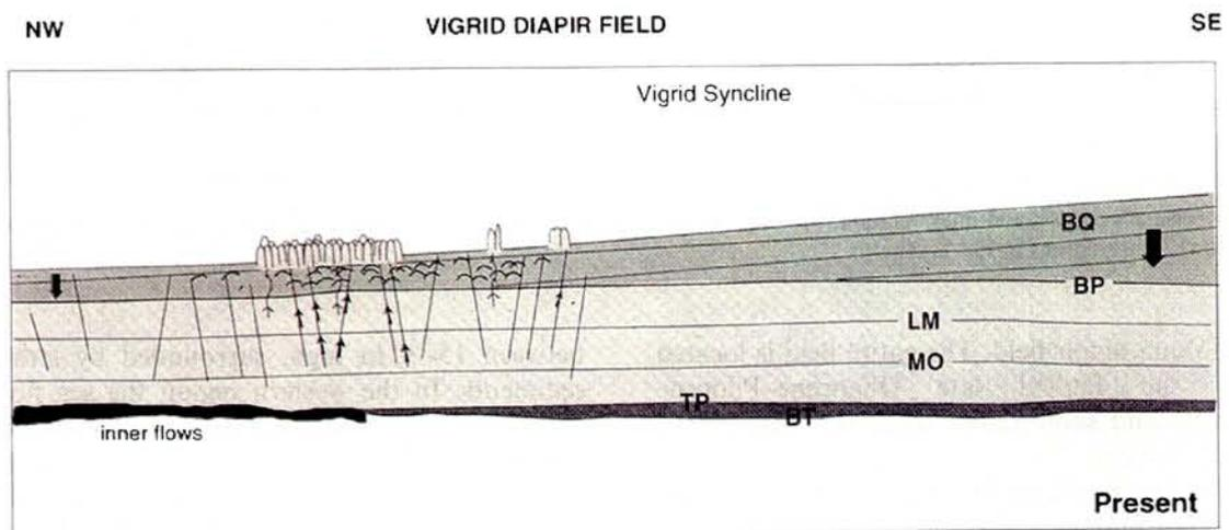
Figure 2.9.2 Geoseismic section through the Vigrid diapir field. After Hjelstuen et al. 1997.
