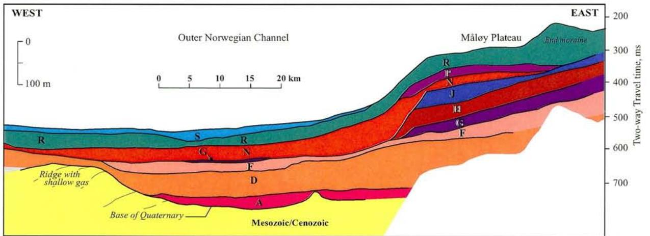
Figure 3.3.4 East-west profile showing the Quaternary stratigraphic units in the Norwegian Channel and the Måløy Plateau at about 62°N (after King et al. in prep).
