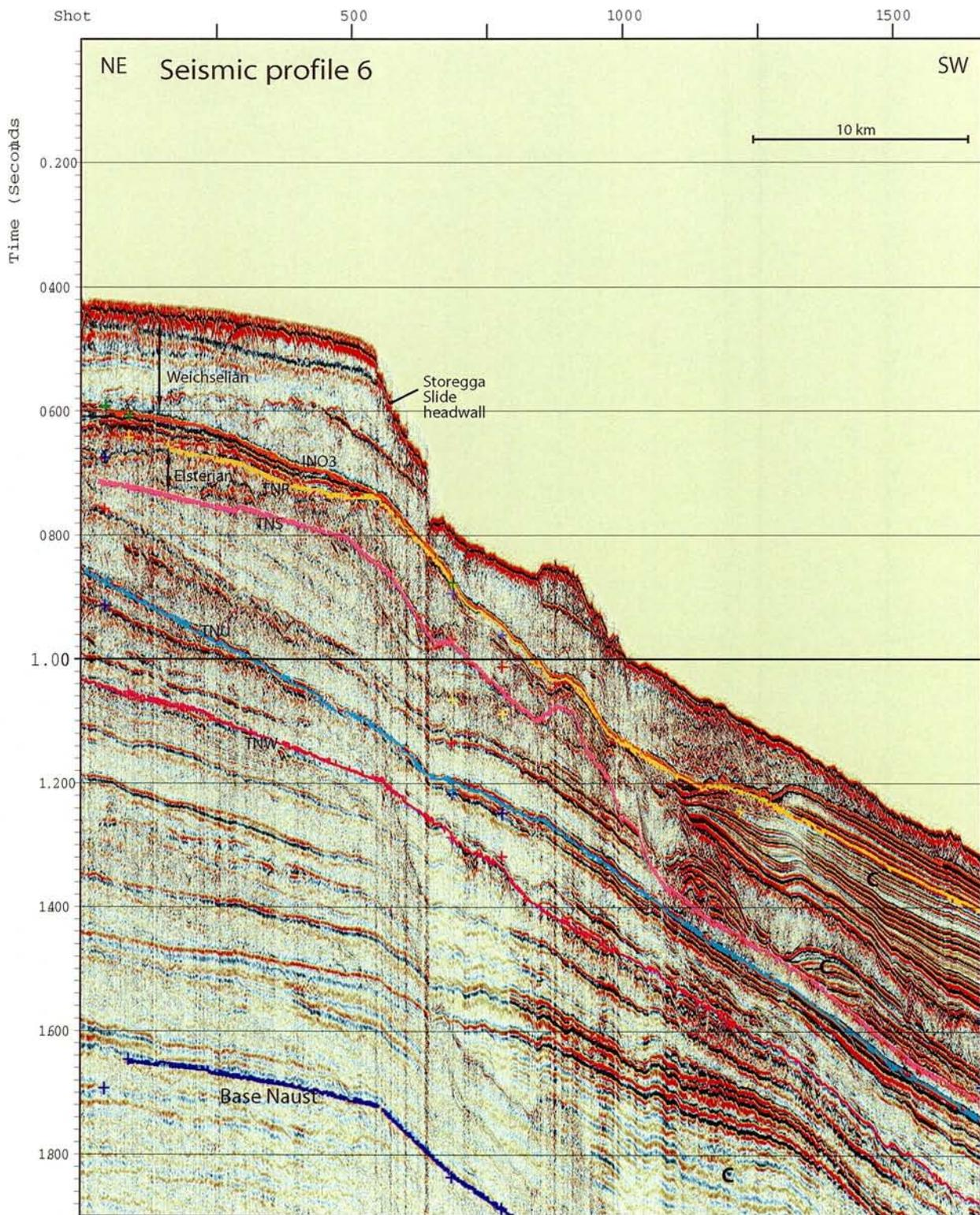
Figure 8.2.3 Seismic profile NH0163-201 from the north-eastern corner of the Storegga Slide and southwestwards. Thick Late Weichselian till deposits occur at the shelf break west of Haltenbanken. Note the slided block, indicating that horizons separating different till tongues may act as glide planes. The mounded contourites ( C ) occur at different intervals. See figure 8.1 for location.
