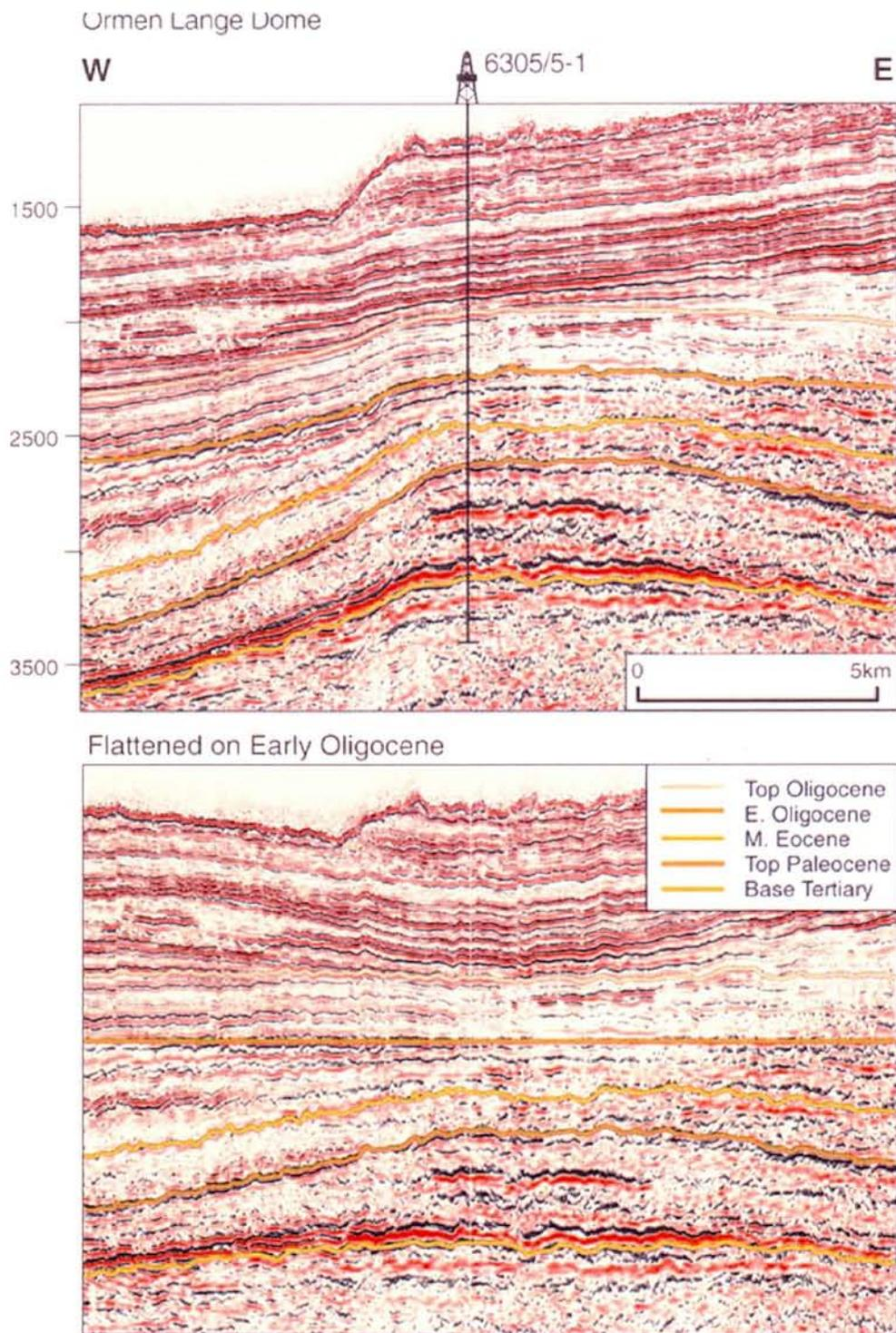
*Figure 2.3.4. Seismic section through the Ormen Lange Dome, illustrating the pulsed nature of compressional doming and the inversion of a Paleocene depocenter. After Lundin and Doré (2002)*
