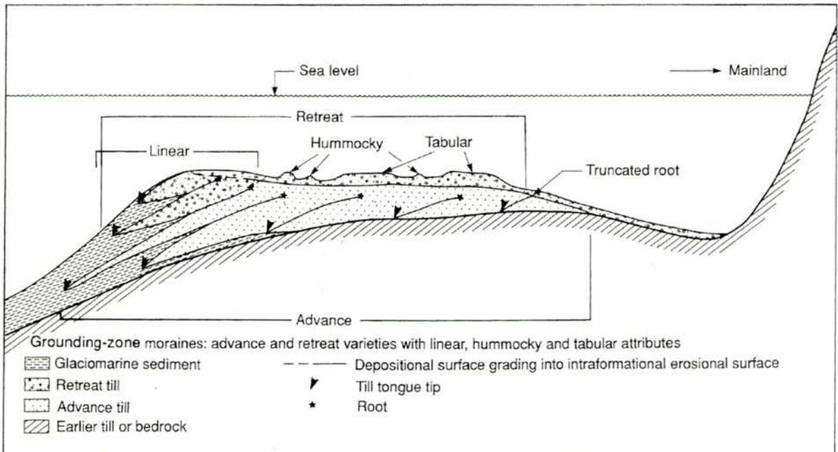
Figure 3.3.9 Diagrammatic section across the mid-Norwegian Shelf, showing the elements of a till tongue stratigraphy during a complete glacial cycle (after King et al. 1991).
