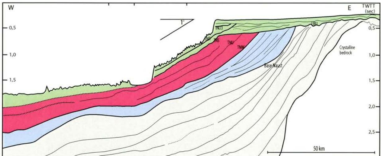
Figure 5.2.5 Line drawing of seismic composite profile 3 from Buadjupet to the Storegga slide area. Blue – Naust W, red – Naust U & S, green – Naust R & O. See figure 5.2.1 for location and table 5.2.1 for reference to applied seismic lines.
