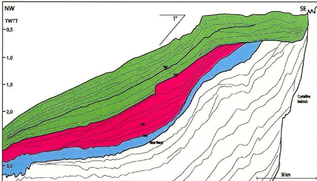
Figure 3 Interpreted seismic profiles showing the main Naust sequences. See Fig. 1 for location. Naust W – blue; Naust U+S – red; Naust R+O – green; Oligocene 'delta' – yellow.
