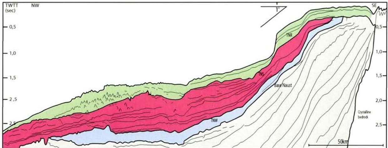
Figure 5.2.4 Line drawing of seismic composite profile 2 from Langgrunna into the Storegga slide area and onto the North Sea Fan. Blue – Naust W, red – Naust U & S, green – Naust R & O. See figure 5.2.1 for location and table 5.2.1 for reference to applied seismic lines.
