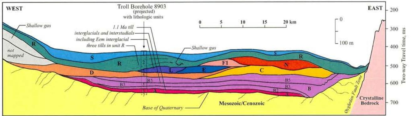
Figure 3.3.1 East-west profile showing the Quaternary stratigraphic units in the Norwegian Channel at about 60° 38' N. Proposed correlation to the Troll borehole 8903 (see Fig. 3.3.2) is marked on the profile (after King et al. in prep.).
