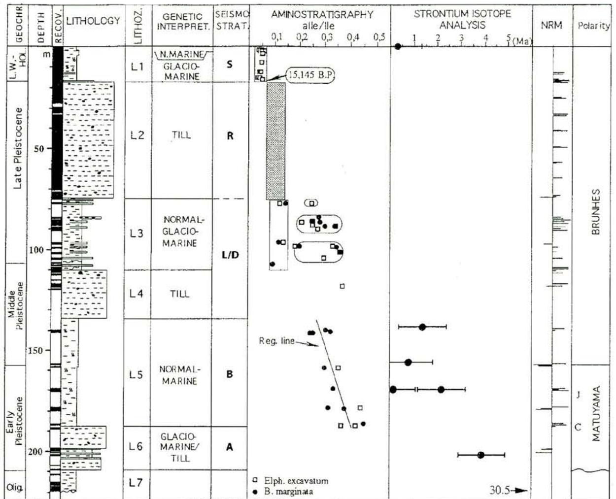
Figure 3.3.2 Chronostratigraphy of borehole 8903 at the Troll Field (after Sejrup et al. 1995).
