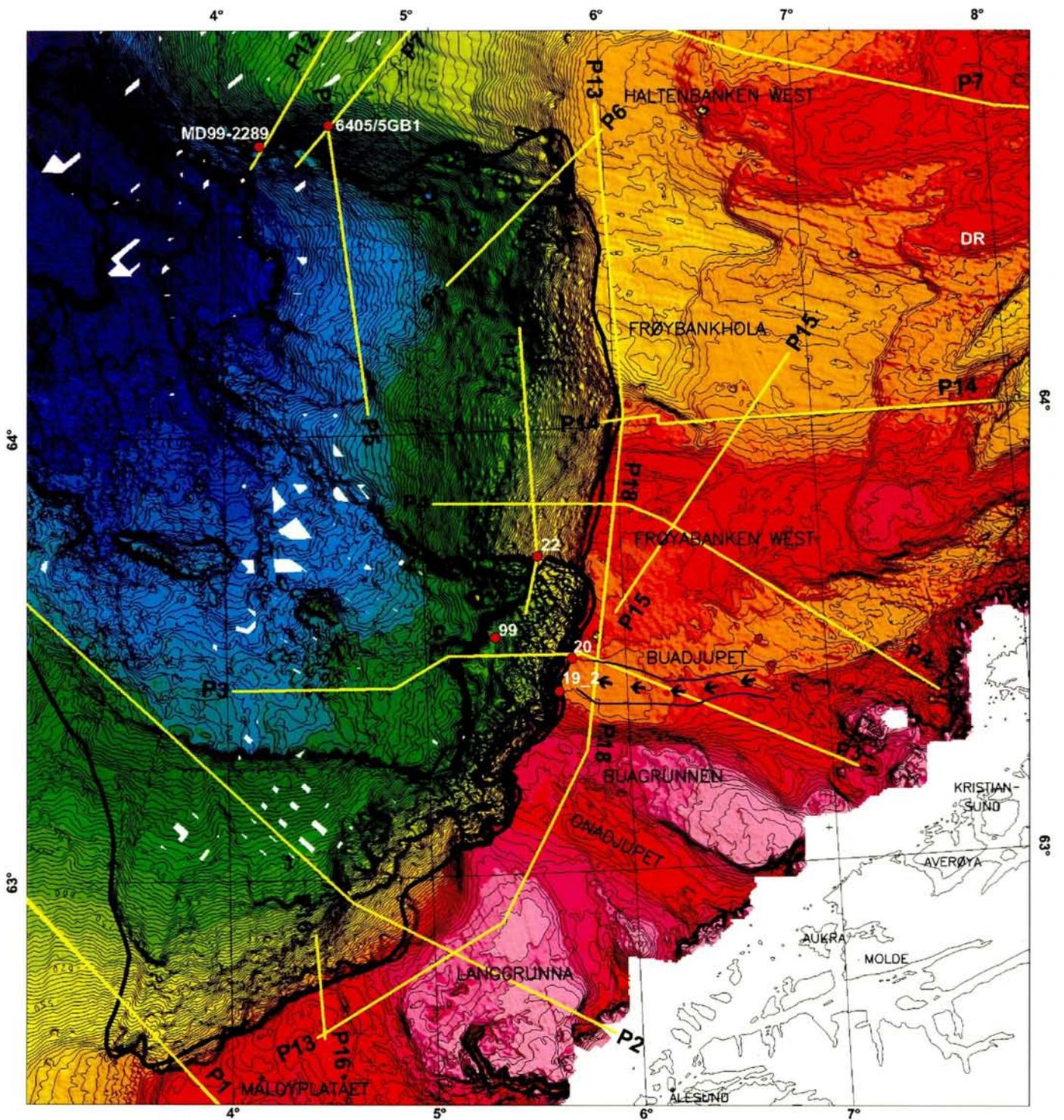
Figure 8.1 Bathymetric map of the eastern part of the Storegga Slide area. Presented seismic profiles and geotechnical boring sites are shown. The arrows mark a buried channel (see Fig. 8.1.1). See table 5.2.1 for reference to the seismic lines applied.
