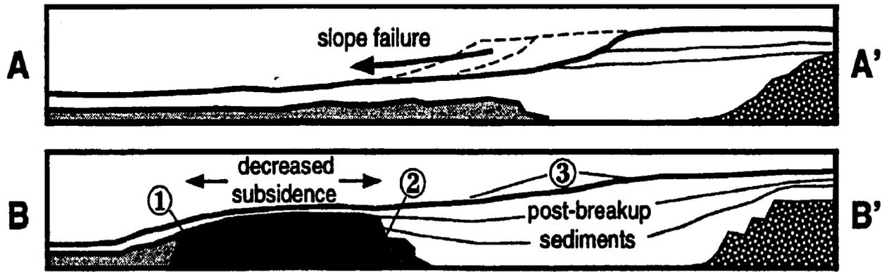
Figure 2.2.5 Idealized cross sections across margin segments without (A) significant underplating and associated marginal high and (B) with significant underplating and associated marginal high. For schematic location see Fig. 2.2.2 Numbers in B-B' suggest influence on slope stability by the magmatic elements: 1) high shear strength of slope material due to shallow buried basalts, 2) barrier against deep-carving slides, 3) small slope angle due to reduced subsidence (From Berndt 2000).
