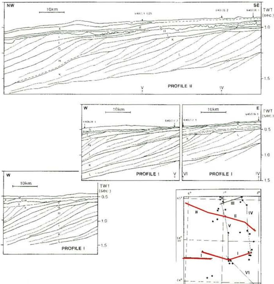
Figure 3.2.2 Geoseismic profiles I and II (red) showing the Late Pliocene/Pleistocene stratigraphic units in the Haltenbanken area (after Rokoengen et al. 1995). Units E, F, G, H, I, K and L comprise prograding subunits of the Naust Formation, while U, A, B and D represent subunits above the Upper Regional Unconformity (URU). Well 6407/9-1 (see profile 1) is located in the Draugen area.
