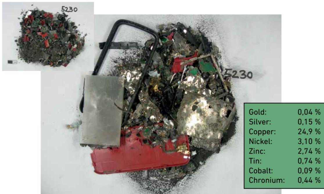
Mobile-phone high technology depends on very many mineral resources. The example above shows a selection of metals, analysed in a crushed Nokia 5230 cell phone.<sup>6</sup>
