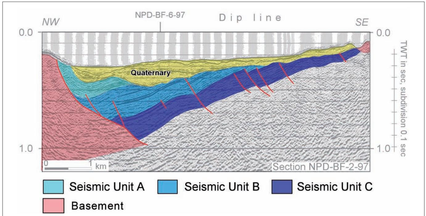
Figure 7. Seismic line, Beitstadfjord Basin. Modified from Sommaruga and Bøe (2002).
