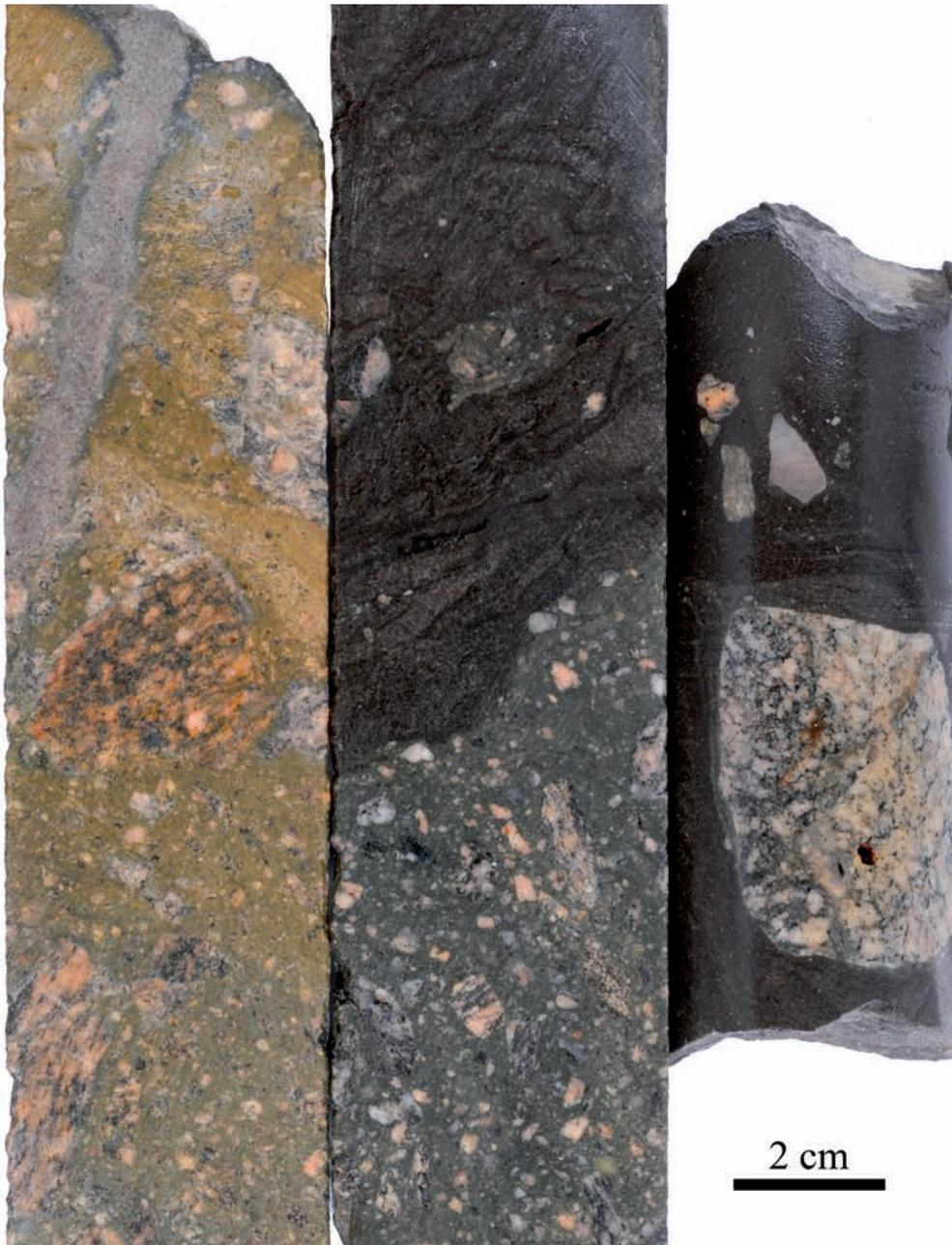
Figure 10. Three core samples of the Mesozoic Bjorøy Formation. Left: Breccia, interpreted as sedimentary, with sand vein (top). Middle: transition from grit to quartz-rich sandstone with a few small coal fragments. Right: sandstone with gneiss fragments. These and other samples from the Bjorøy tunnel in West Norway are part of the Natural History Collections at Bergen Museum, University of Bergen.
