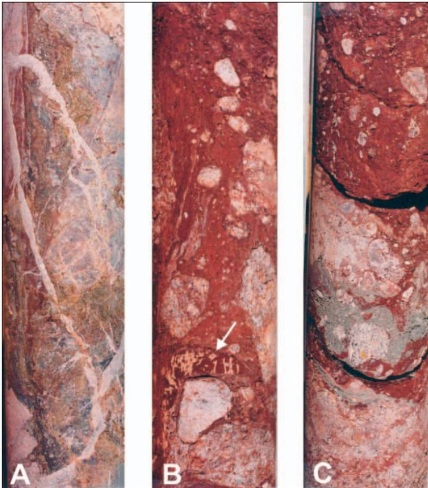
Fig. 4. Details of breccias in core BH2 (see Fig. 2 for location) from (A) c. 46.3 m, (B) 52.5 m and (C) 75 m depths. Core width is c. 7 cm. (A) Calcite-cemented and calcite-veined gneiss/fault breccia. (B) and (C) Matrix-rich, sediment- and gneiss-bearing fault breccias. Note the dolomite-veined fragment in the lower part of B (arrow).
