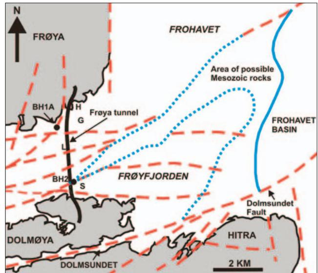
Fig. 2. Tectonic lineaments interpreted from bathymetry and aerial photographs in the Frøyfjorden area (modified from Sættem & Mørk 1996). The location of the Frøya tunnel, boreholes BH1A and BH2 and major fault and fracture zones (dashed lines) are shown. H: Hammarvik; G: Grønholman; L: Løkskjæra; S: Seibalskjæra. See Fig. 1 for location. The western border of the Frohavet Basin is indicated by the continuous blue line.
