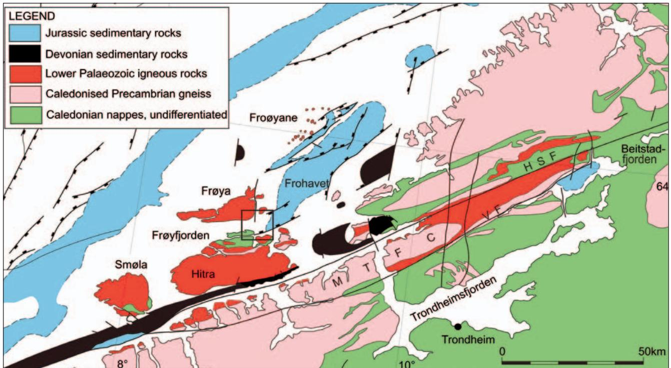
Fig. 1. Geological overview map. Subcropping Jurassic rocks are shown in blue colour. Devonian rocks on land and below the sea are shown in black. MTFC – Møre-Trøndelag Fault Complex; HSF – Hitra-Snåsa Fault; VF – Verran Fault.
