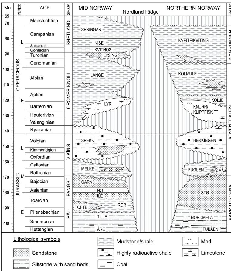
Fig. 2. Time correlation of stratigraphic formations offshore Mid-Norway (Dalland et al. 1988) and Northern Norway (Worsley et al. 1988, Smelror et al. 2001b). Based on Mørk et al. (2003).
