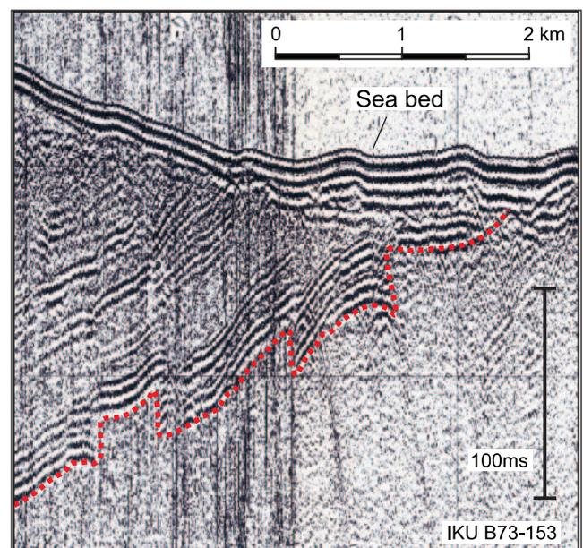
Fig. 5. Shallow seismic (sparker) section showing the block-faulted reflector forming the border between Units IV and V (red dots). For location, see Fig. 3.
