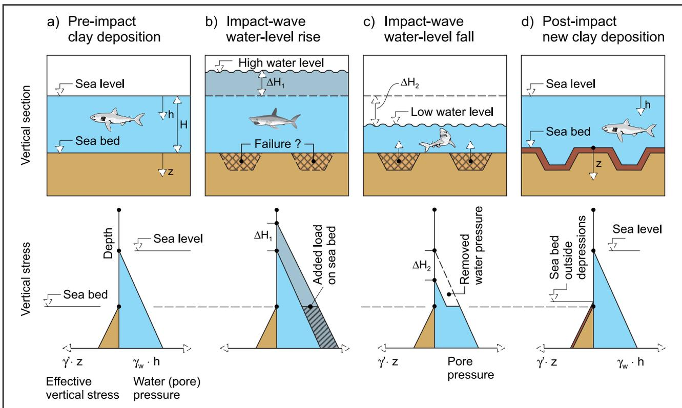
Fig. 8. Simplified two-dimensional, geotechnical explanation model for the formation of the irregular base Cretaceous reflector offshore Mid Norway. See text for more details about the different cases.  $\gamma$  – dry unit weight of soil (kN/m<sup>3</sup>);  $\gamma_w$  – unit weight of water (kN/m<sup>3</sup>);  $z$  – depth below sea bed;  $H$  – original water depth;  $h$  – depth below sea level;  $\Delta H_1$  – impact water level rise;  $\Delta H_2$  – impact water level fall
