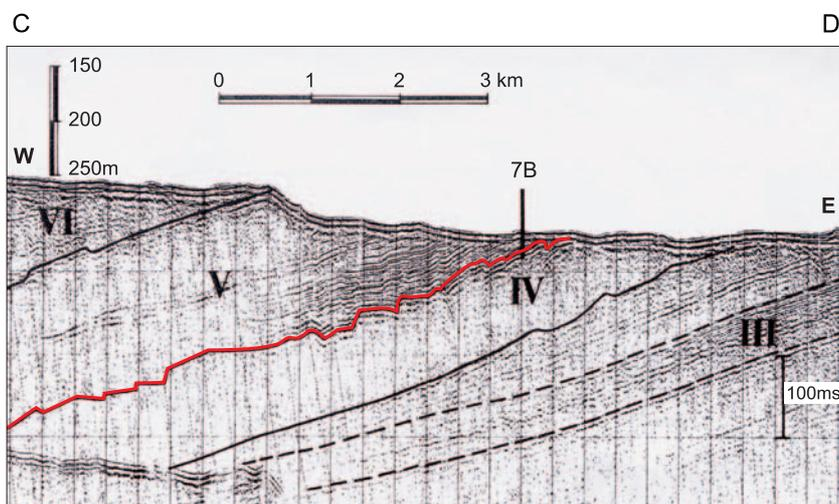
Fig. 6. Shallow seismic (sparker) line IKU B78-103 with location of borehole 7B. Location shown in Fig. 4. The border between Units IV and V is marked in red. After Mørk et al. (1983) and Århus et al. (1986).
