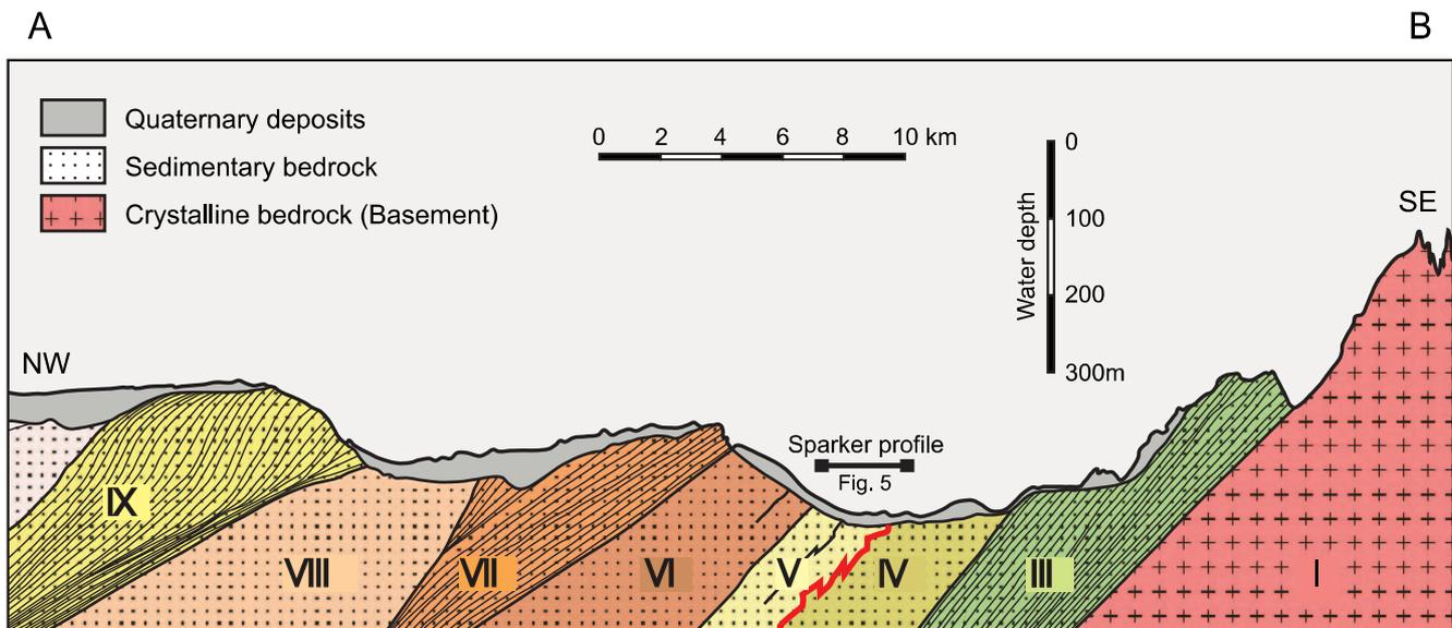
Fig. 3. Geoseismic section (line IKU B73-153) showing the shallow bedrock geology offshore Mid Norway. Approximately 30x vertical exaggeration. Location shown in Fig. 4. Modified from Bugge et al. (1976, 1984). The units I to XI are described in the text and the assumed Jurassic-Cretaceous boundary (contact between Units IV and V) is marked in red.
