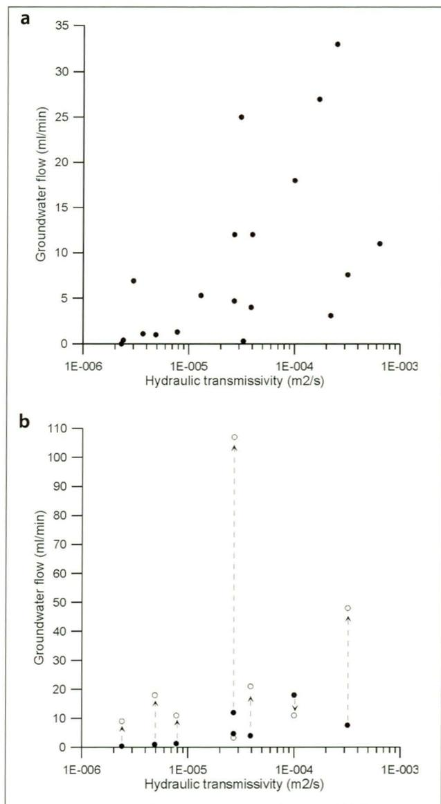
Fig. 15. Groundwater flow versus hydraulic transmissivity; (a) All borehole sections measured during undisturbed natural hydraulic gradient conditions. (b) Flow during a large-scale pumping test, LPT-2, (circles) compared to natural gradient conditions (dots).
