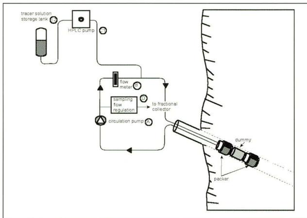
Fig. 6. Dilution equipment for application in tunnels.
