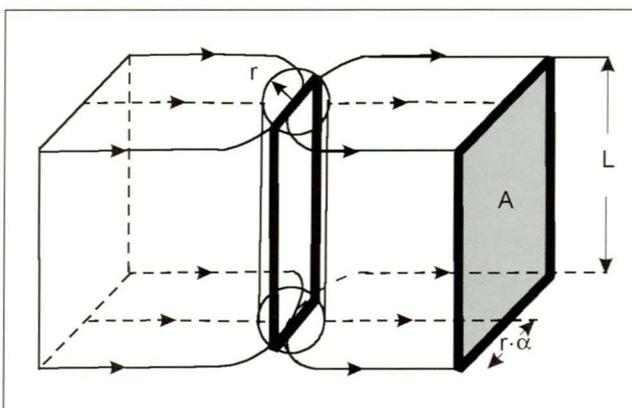
Fig. 2. Flow lines in the vicinity of the borehole test section in the ideal case.
