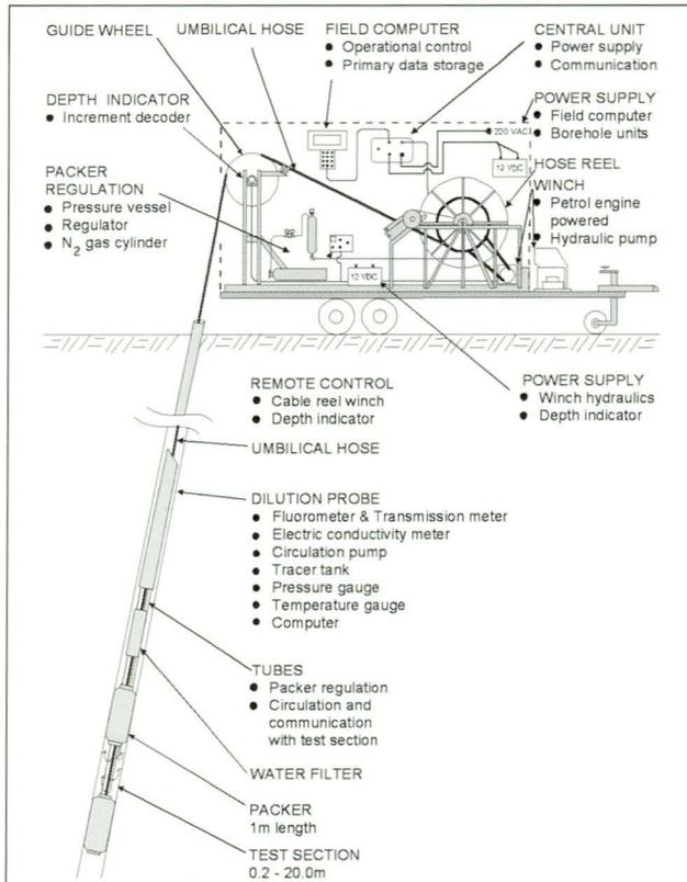
Fig. 4. The Borehole Probe Dilution Equipment.
