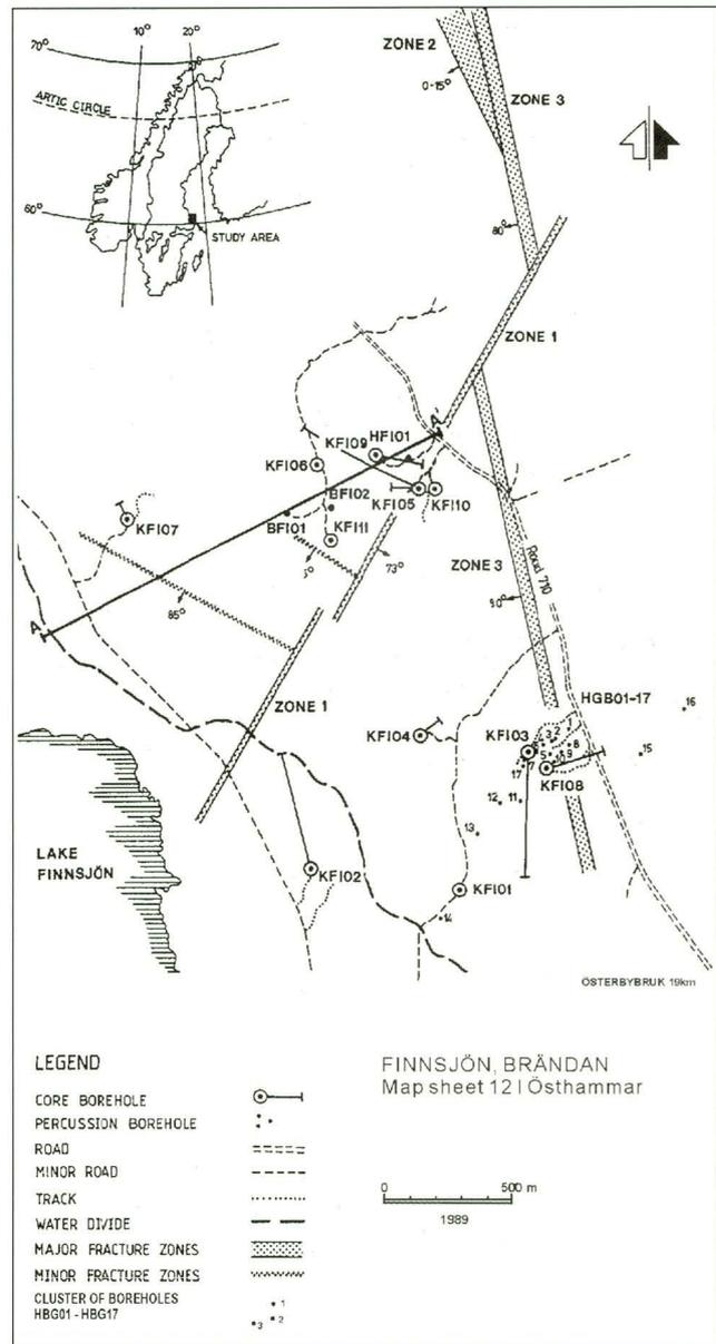
Fig. 7. Map of the Finnsjön site showing borehole locations and major fracture zones. Section A-Å illustrated in Fig. 9 is also marked.
