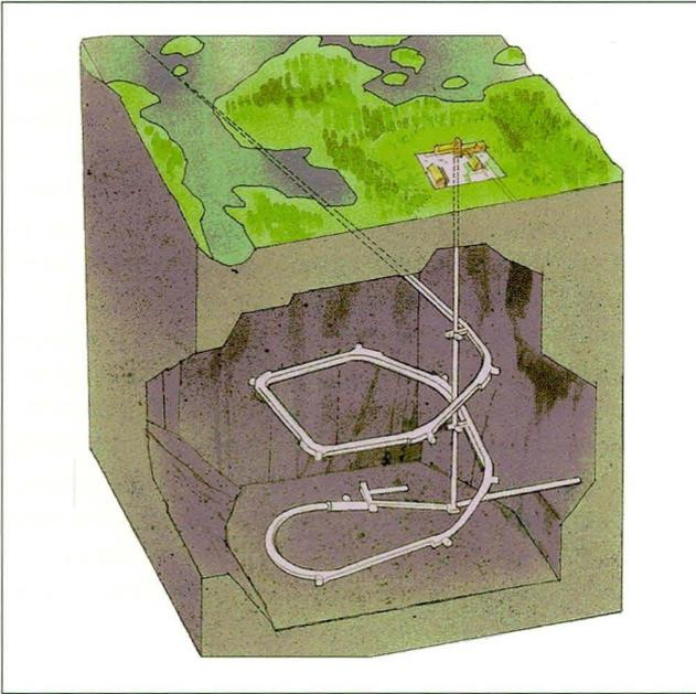
Fig. 13. General layout of the Äspö Hard Rock Laboratory, with a total tunnel length of 3600 m and maximum depth 450 m.
