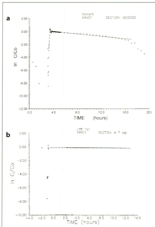
Fig. 17. Examples of dilution curves from measurements in borehole KAV01; (a) High groundwater flow rate (31.5 ml/min) in a shallow, highly conductive, fracture zone. (b) A low conductive fracture at depth with a low flow rate (0.008 ml/min).
