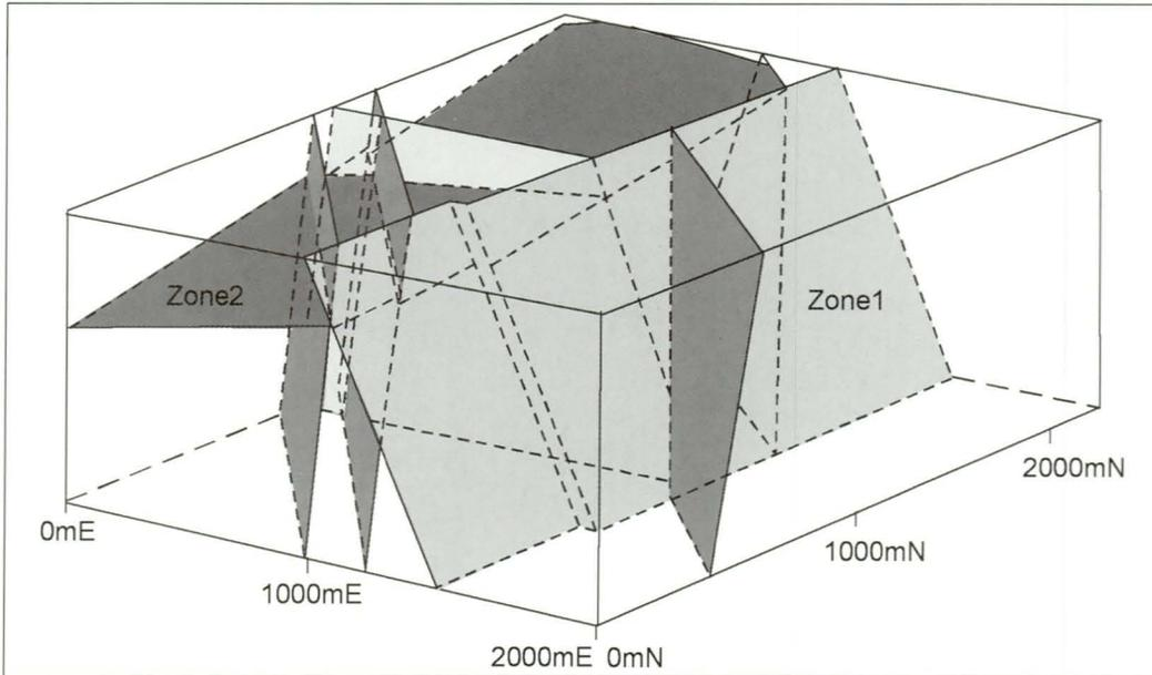
Fig. 8. Conceptual model of the fracture zones in the Brändan area, Finnsjön site.
