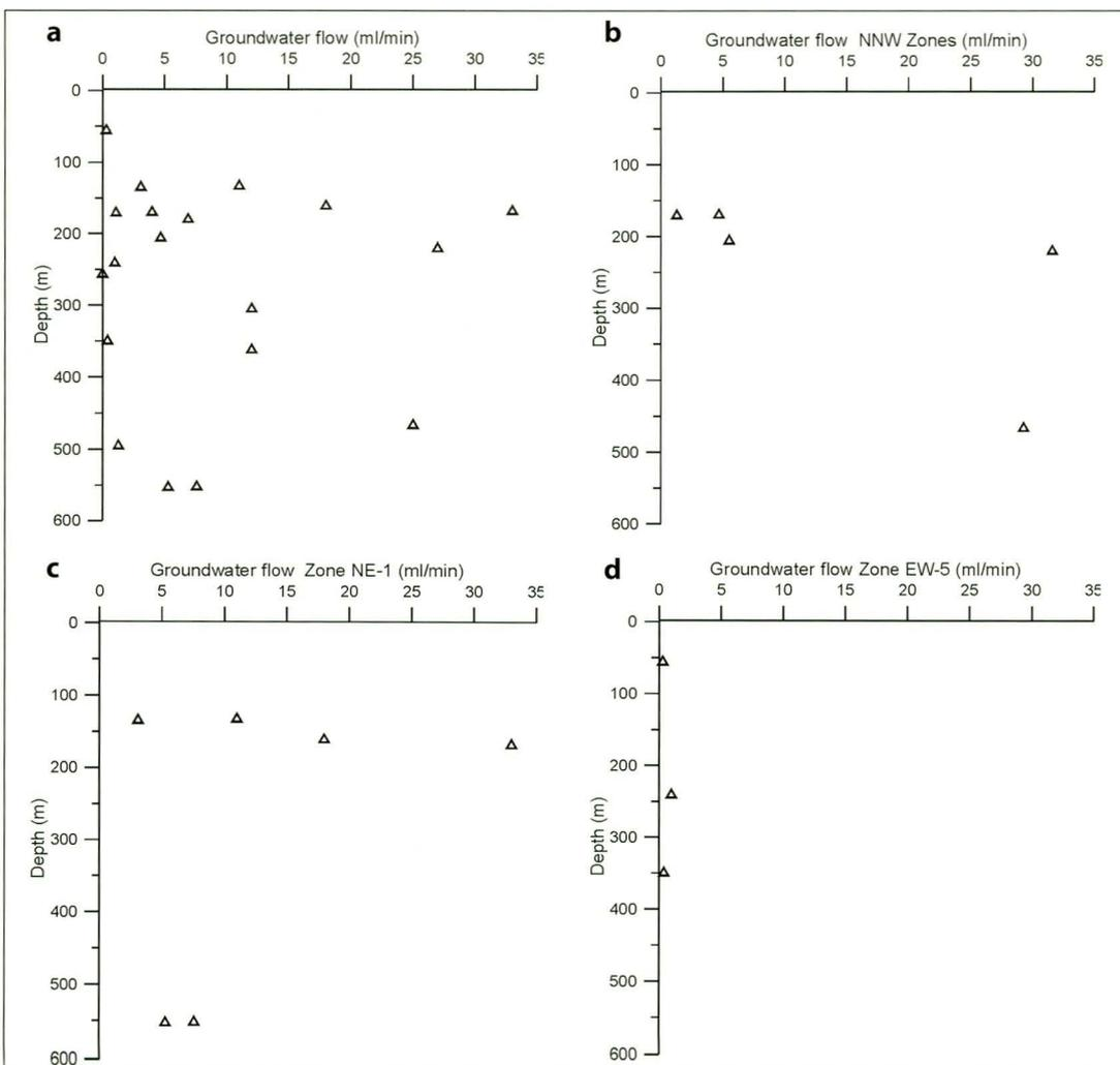
Fig. 14. Groundwater flow versus depth during undisturbed natural hydraulic gradient conditions; (a) All borehole sections measured. (b) Flow in the NNW-SSE orientated fracture zones NNW, NNW-1 and NNW-2. (c) Flow in the NE-SW orientated fracture zone NE-1. (d) Flow in the E-W orientated fracture zone EW-5.
