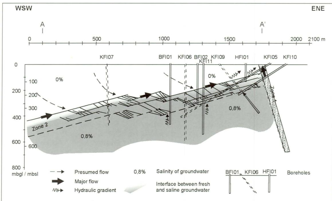
Fig. 9. Transverse hydrogeological section A-A' (see Fig. 7 for location).
