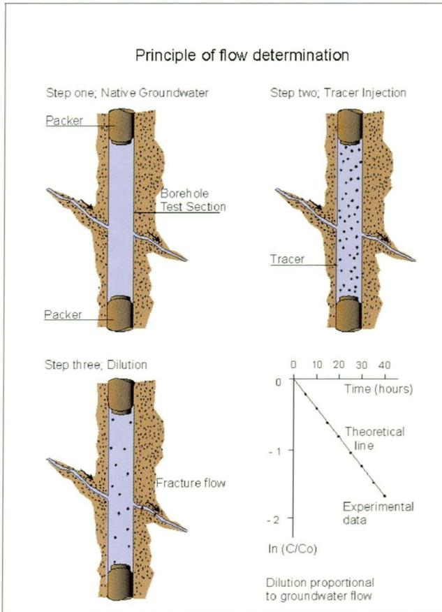
Fig 1. Principle of flow determination by the dilution method.
