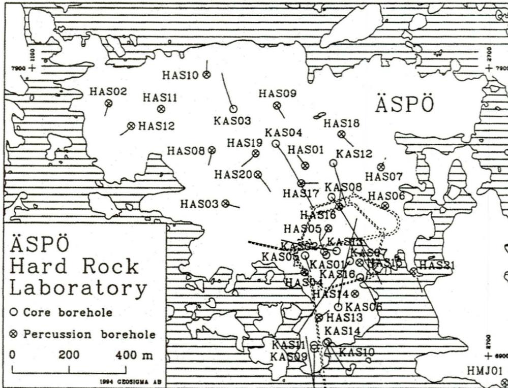
Fig. 12. Äspö with borehole locations. Circles represent the intersections of the boreholes with the ground surface, the lines represents the projection on the ground surface of the borehole. The HRL tunnel excavation is also indicated (dotted lines).
