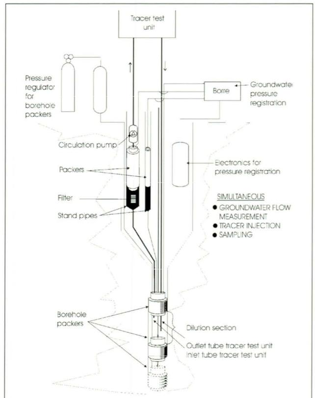
Fig. 5. Principle of the Multipacker system, equipped for groundwater flow measurements by the dilution method.
