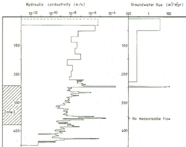
Fig. 10. Results of groundwater flow measurements by the dilution method in borehole BFI01 compared with the hydraulic conductivity, determined from hydraulic injection tests.
