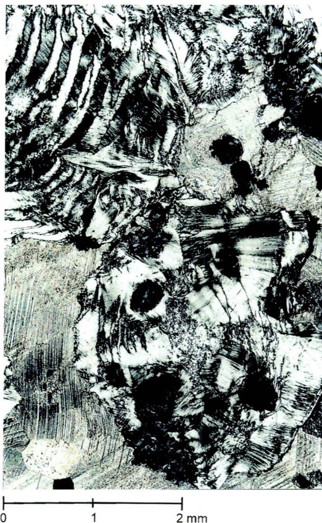
Fig. 4. Brucite as a series of concentric swirls of foliated aggregates. The bluish/black enclosed grains are fragments of unaltered forsterite. Photomicrograph under crossed nicols.
