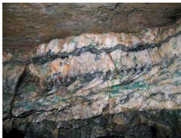
Figure 20. Left: Molybdenite along the contact between pegmatitic quartz vein and granite in the Bandaksli deposit. Right: Molybdenite and bornite in a 15-cm-wide quartz vein in greenstone at the Askom mine (diameter of the coin is 22 mm). Photos: J. S. Sandstad, NGU.
