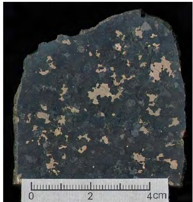
Figure 12. Pyrrhotite-pentlandite ore in peridotite at Stormi. Scanned image by Hannu Makkonen, GTK.
