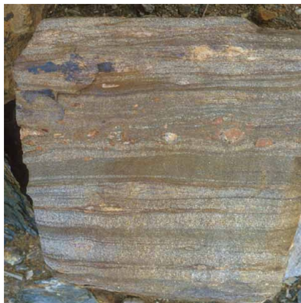
Figure 44. A mineralised block from the Vingelen deposit, showing primary banded ore with light pyrite-chalcopyrite bands alternating with dark sphalerite-pyrite bands. Size of block approximately 50 x 50 cm. Photo: T. Bjerkgård, NGU.
