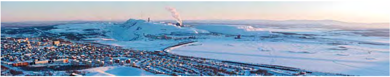
Figure 34. Panoramic view of the Kiruna iron ore deposit looking south. The outcropping iron ore (all exploited) was located on the eastern (left) side of the mountain in the left-centre part of the photo. The iron ore dips steeply (60–70°) to the east (left) under the town of Kiruna. The plume of smoke in the centre of the image comes from the pelletisation plant. Copyright: LKAB.
