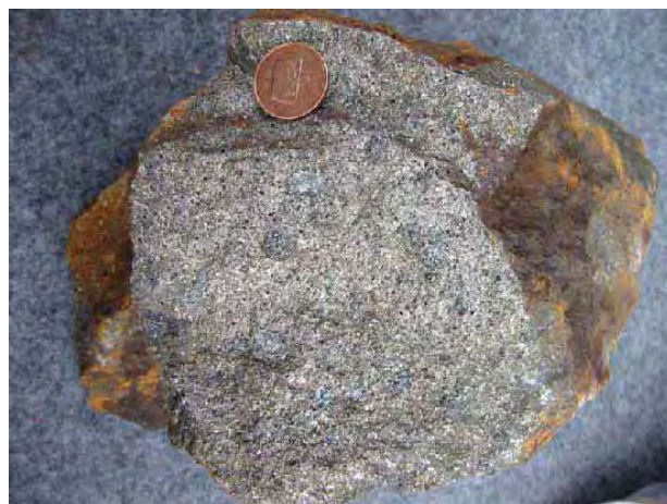
Figure 17. Grab sample of massive ore containing 5.05% Cu, 0.15% Ni and 0.15% Co from the Vissestad waste dump. Diameter of the coin is 18.5 mm. Photo from http://www.blv.ca/s/Bamble.asp .
