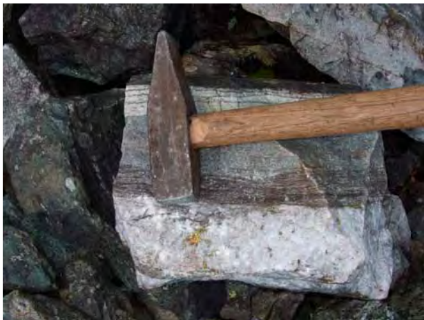
Figure 21. Upper photo: the dumps of the closed Åmdal mine. The ore zone continues up the hill to the left. Lower photo: chalcopyrite aggregates in a quartz vein in quartz schist at Åmdal mine. Photos: J. S. Sandstad and T. Bjerkgård, NGU.
