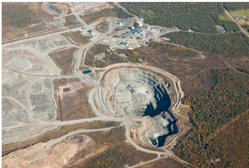
Figure 86. Aerial view of the Suurikuusikko (Kittilä) mine site in September 2010. The ore zone is visible as a dark grey band in the middle of the main open pit. The small Rouravaara open pit is at upper left. View to the NE. Photo: courtesy of Agnico-Eagle Mines Ltd.
