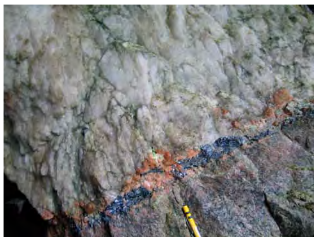
Figure 20. Left: Molybdenite along the contact between pegmatitic quartz vein and granite in the Bandaksli deposit. Right: Molybdenite and bornite in a 15-cm-wide quartz vein in greenstone at the Askom mine (diameter of the coin is 22 mm). Photos: J. S. Sandstad, NGU.
