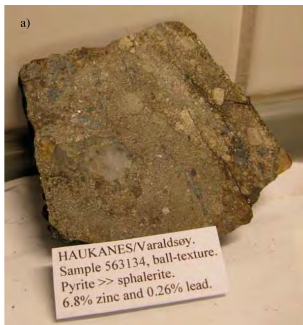
Figure 33. Typical ore samples from the Hardanger district. a) Pyrite-zinc ore from Haukanes deposit. b) Banded magnetite-pyrite ore from Dyråsen. Photos: P. Wulff; the labels are 5 cm long.
