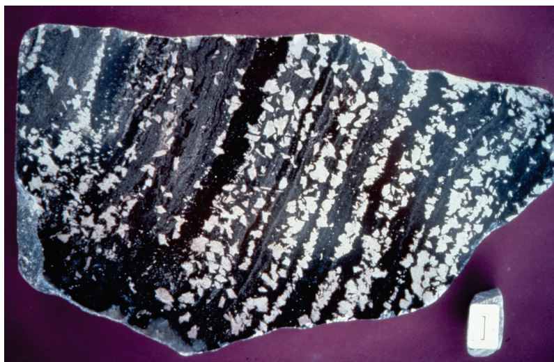
Figure 2. Lupin: iron formation-hosted stratabound gold. Arsenic-rich gold-bearing sulphide iron formation showing sulphide-arsenide megacrysts distributed along bedding. Scale bar is 1 cm. GSC 1995-201A;
