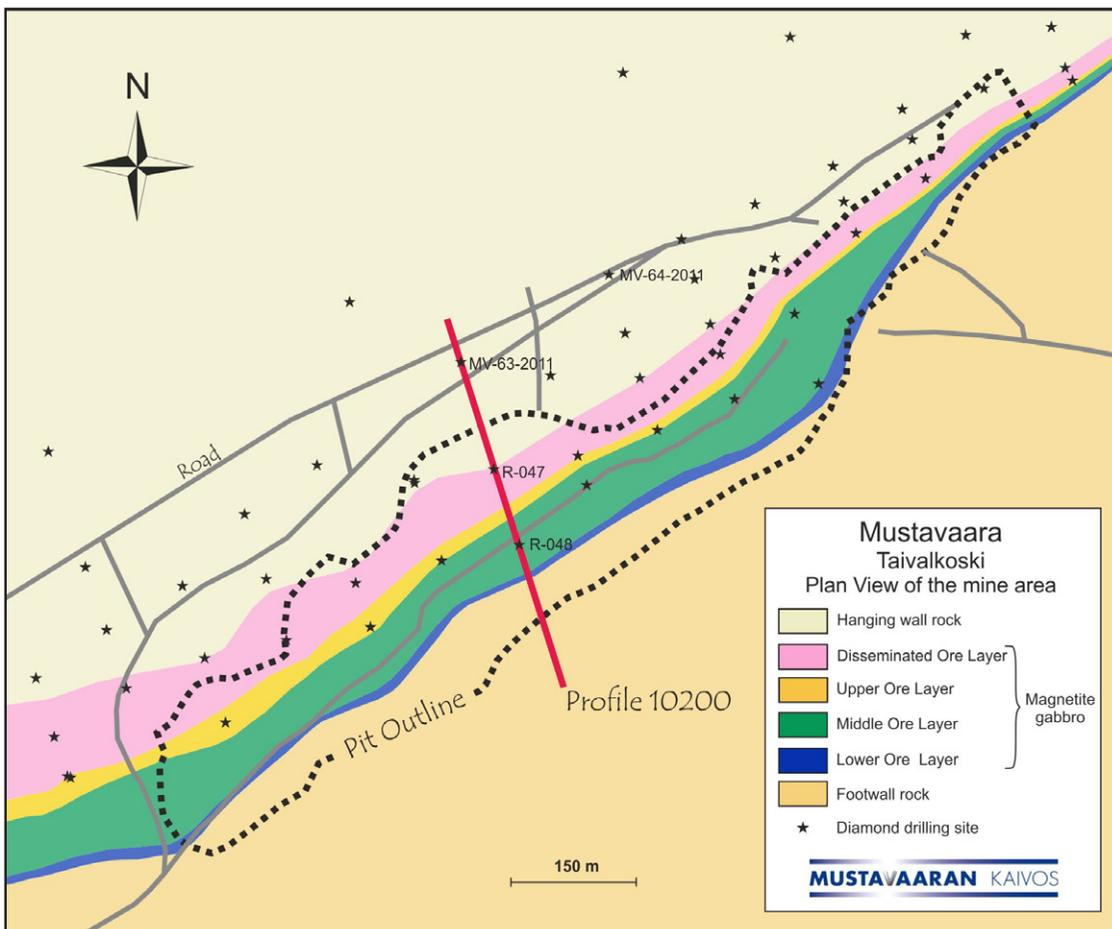
Figure 22. Plan view of the Mustavaara open pit area showing the ore layers projected to surface.
