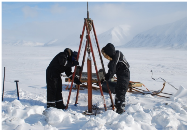
Coring (pisotn corer) the tidal sediments
