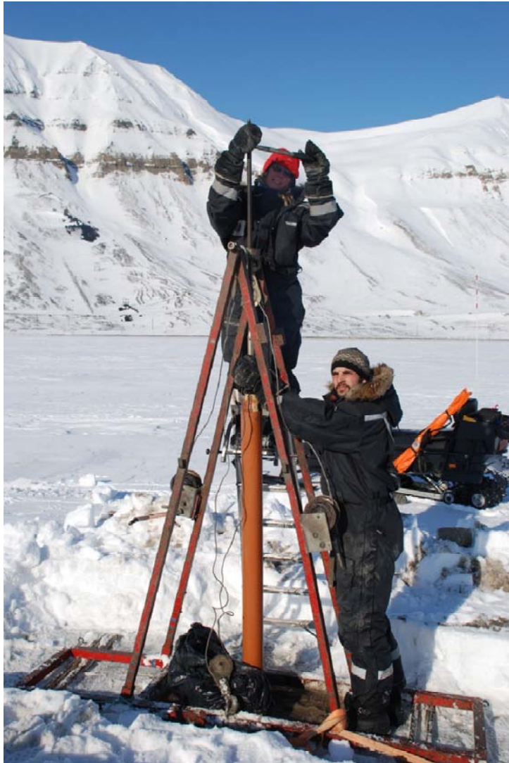
Coring tidal sediments at Braganzavågen
