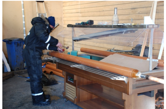
Sampled sediment core is sealed
