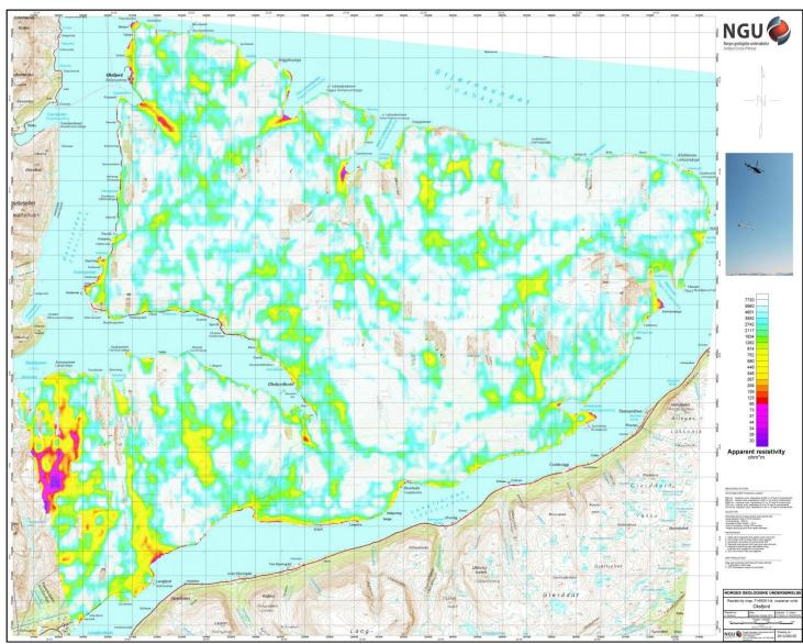
Figure 8: Apparent resistivity. Frequency 6600 Hz, Coplanar coils
