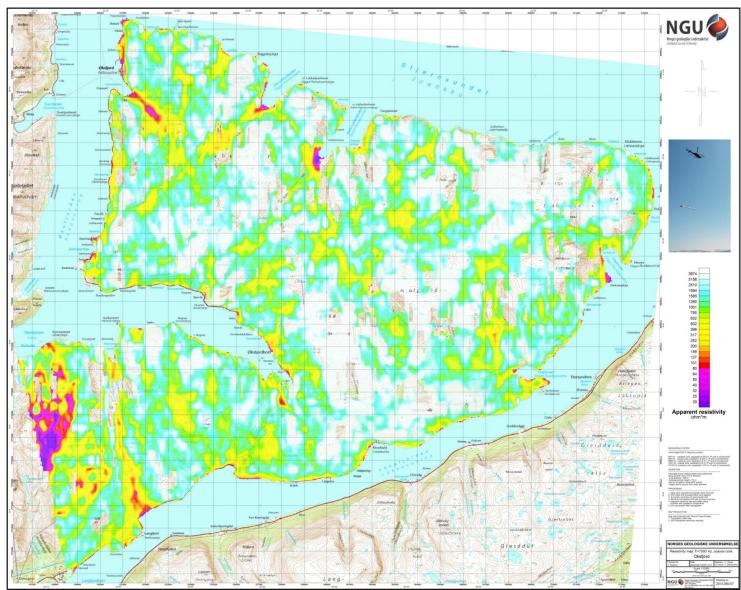
Figure 10: Apparent resistivity. Frequency 7000 Hz, Coaxial coils
