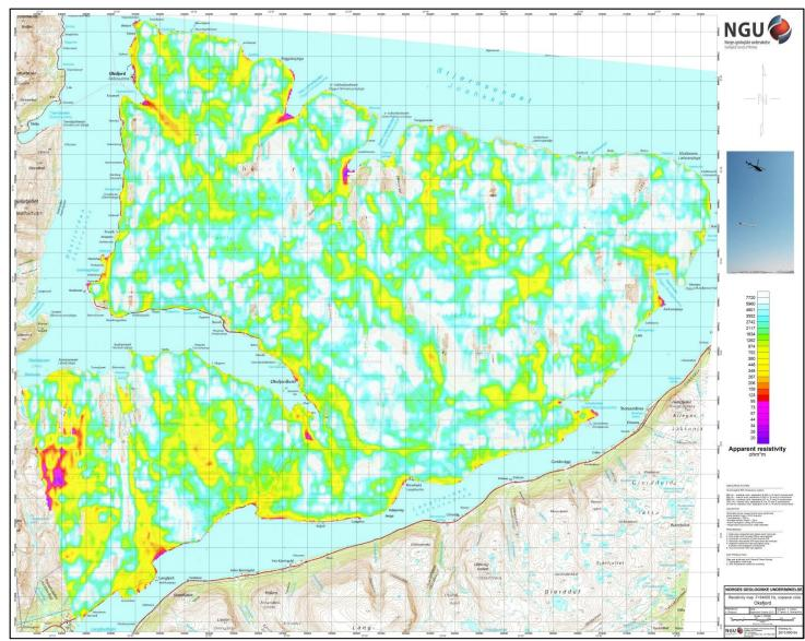
Figure 7: Apparent resistivity. Frequency 34000 Hz, Coplanar coils
