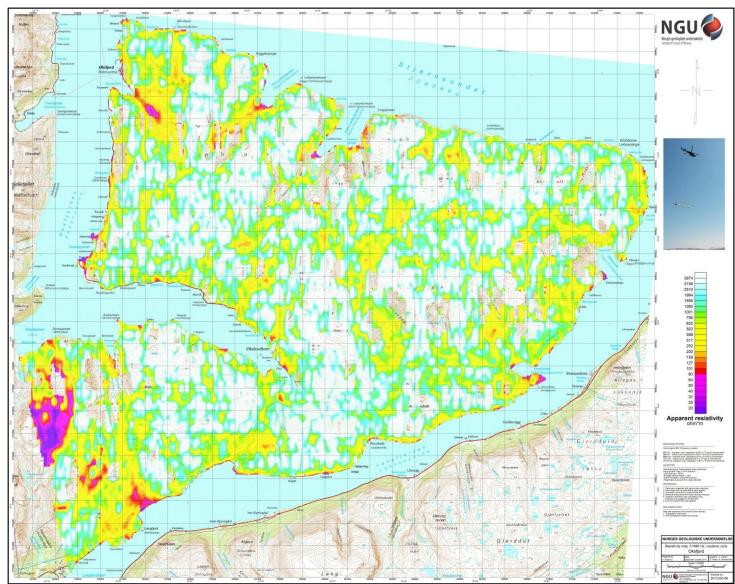
Figure 9: Apparent resistivity. Frequency 880 Hz, coplanar coils
