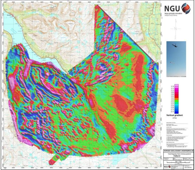
Figure 6: Magnetic Vertical Derivative
