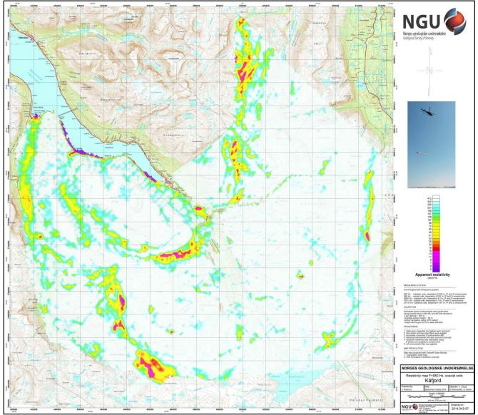
Figure 11: Apparent resistivity. Frequency 980 Hz, Coaxial coils
