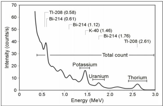
Figure 3: An example of Gamma-ray spectrum showing the position of the K, Th, U and Total count windows (Peak energy in bracets).
