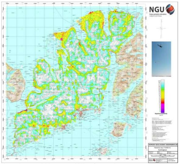
Figure 7: Apparent resistivity. Frequency 34000 Hz, Coplanar coils
