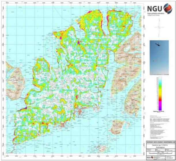
Figure 3: Apparent resistivity. Frequency 7000 Hz, Coaxial coils
