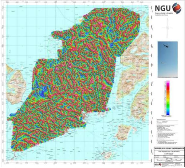
Figure 6: Magnetic Tilt Derivative
