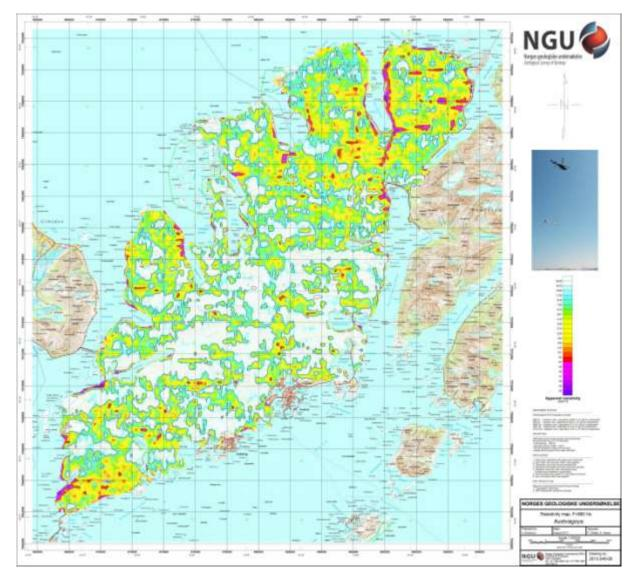
Figure 4: Apparent resistivity. Frequency 980 Hz, Coaxial coils
