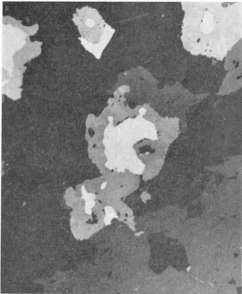
Fig. 11. Ilmenite with corona of sphene (reflection pleochroism). Storelv. Magnif. 90 ×.
