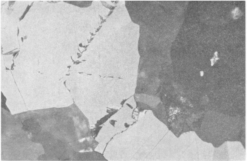
Fig. 7. Rutile (light grey) and sphene (dark grey rim) after ilmenite. Breivikbotn. Magnif. 330 \times . Oil immersion.
