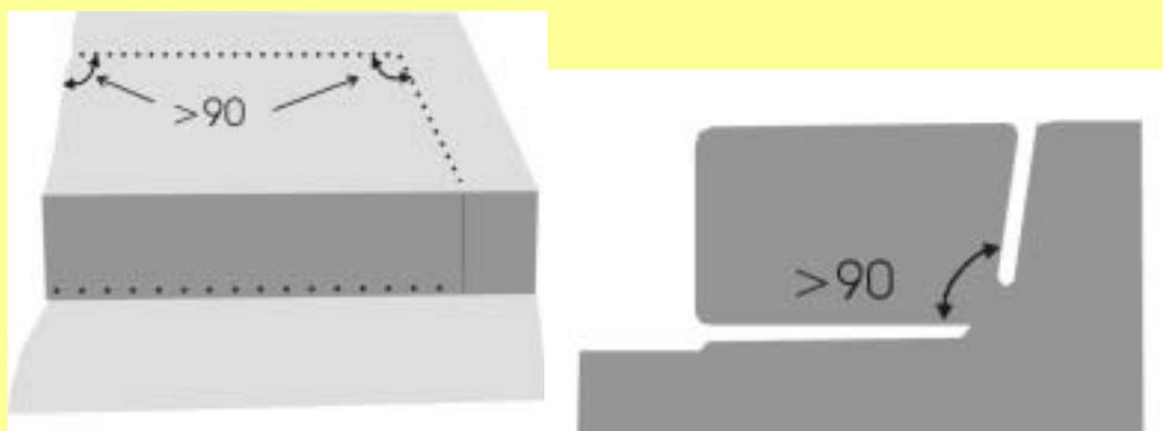
*Illustration of the "Finnish method" in granite quarrying. Front view (left) and cross section through a primary block (right).*
