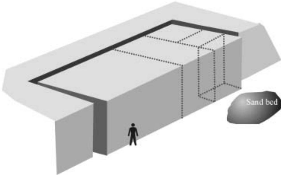
*Principle of block extraction – from primary blocks to smaller sized slices, which will be further divided to commercial blocks.*
