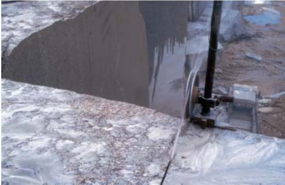
*Diamond wire sawing in a granite quarry, Spain*
