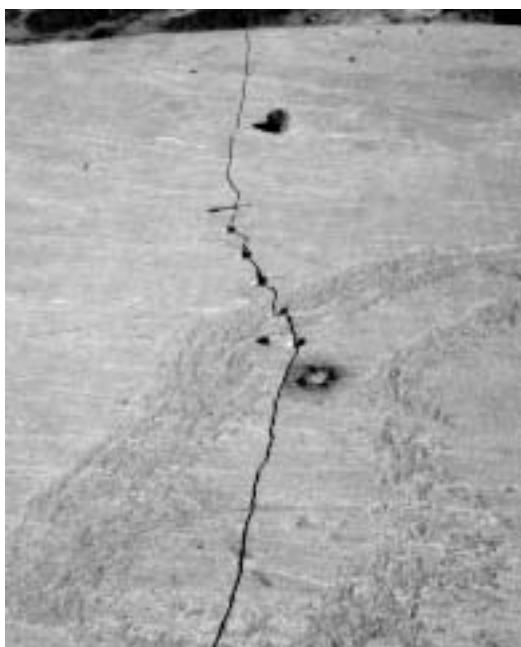
*An example where direction of blasting (row of drill holes) did not correspond with the natural, secondary cleavage (“grain”) in a granite. The cut followed the latter.*
