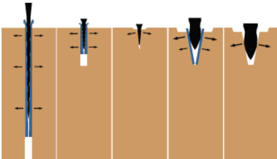
*Principles of wedging. From left to right: long "plug and feather" and penetrating drill holes, short "plug and feather" in short drill holes, short plug in chiselled groove, and finally two examples with large wedges.*
