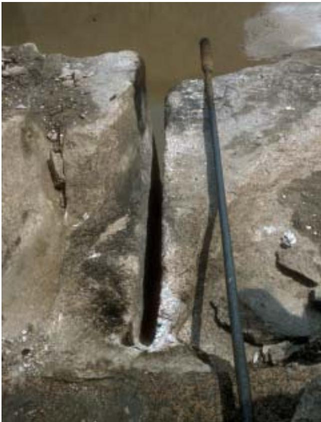
*Channel from jet-burning in granite quarry, and jet-burner (right).*
