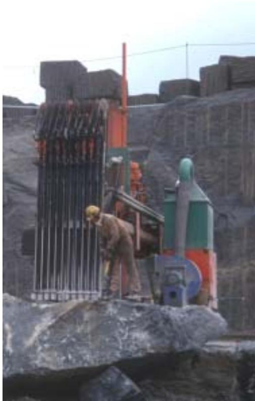
*Multi-hammer, hydraulic driller for squaring of blocks.*
