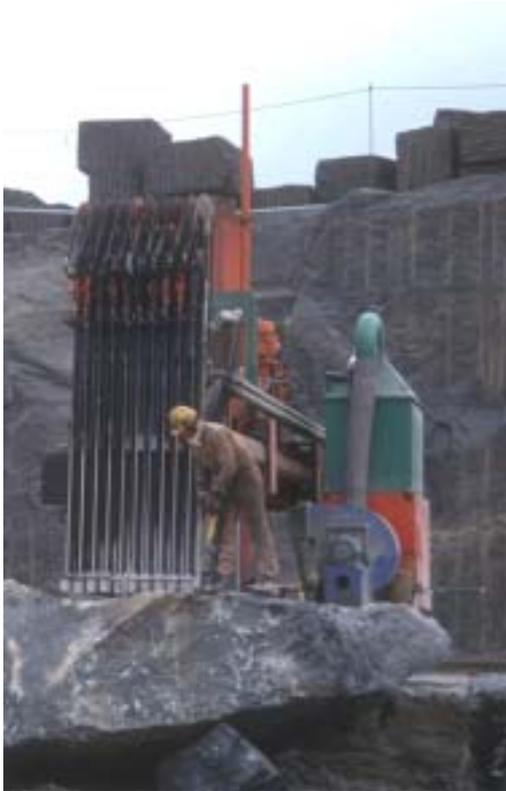
*Multi-hammer, hydraulic driller for squaring of blocks.*
