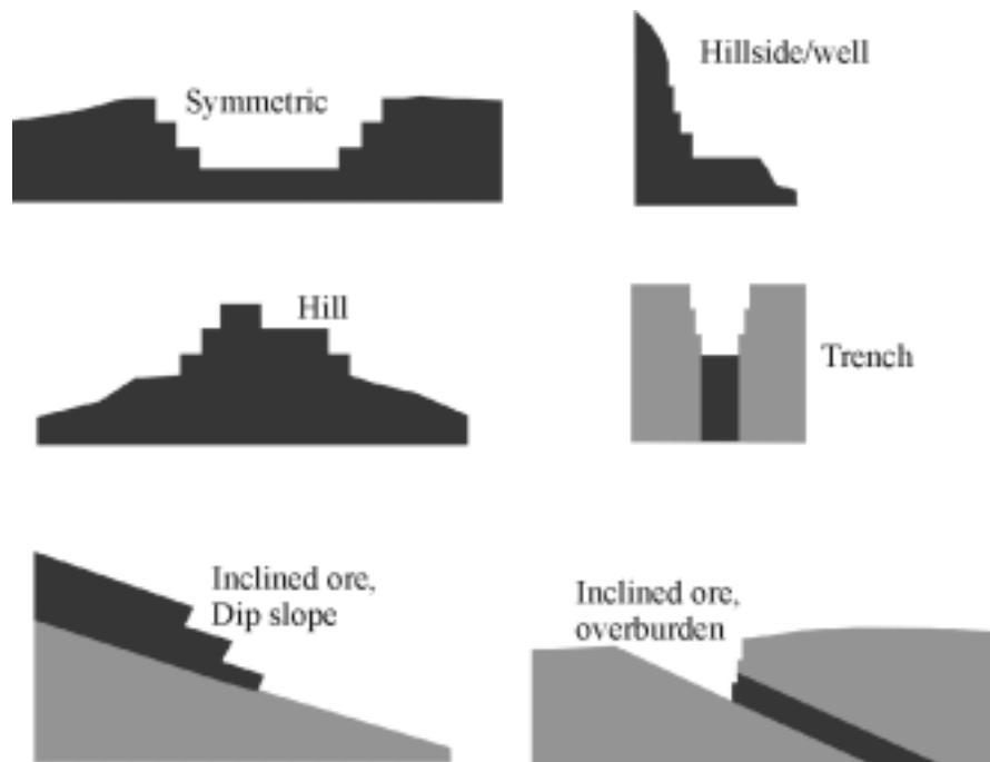
*Schematic drawing showing some different open-cast situations. Workable part of deposit shown in black.*
