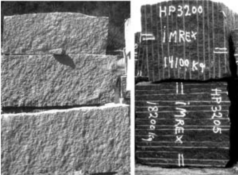
*Rough granite blocks squared with short wedges (left) and long "plugs and feathers". The former granite is far more brittle and easier to split than the latter.*
