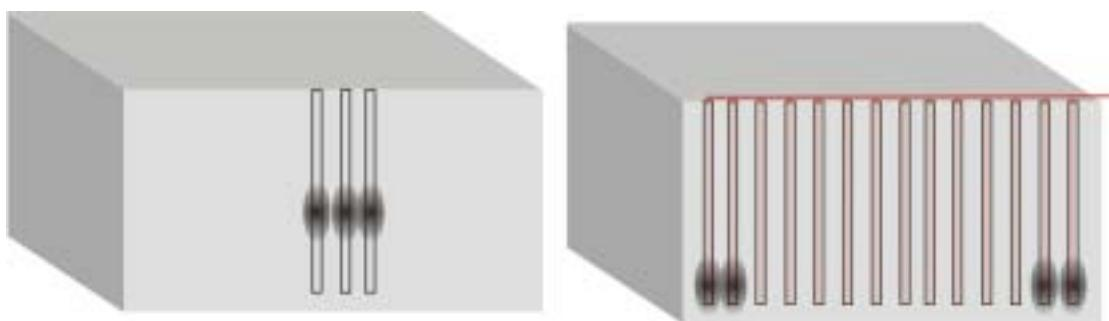
*Two examples of granite splitting with the use of black powder. Left: black powder (dark spots) in three central holes placed along the primary cleavage plane of the granite. Right: black powder only in the marginal holes, combined with detonating fuse (red line)*
