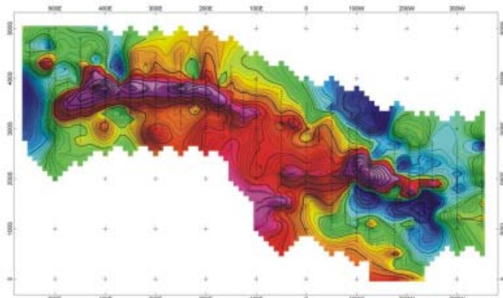
*Ground magnetic survey for tracing the extension of a soapstone deposit beneath soil cover. Violet colour marks the soapstone formation. Grid in metres.*
