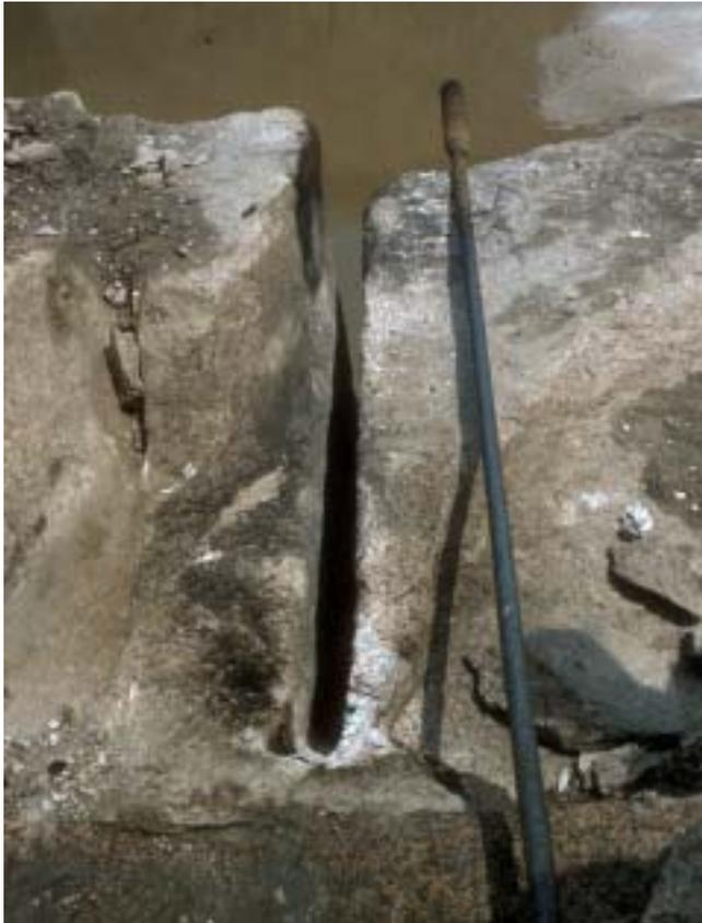
*Channel from jet-burning in granite quarry, and jet-burner (right).*
