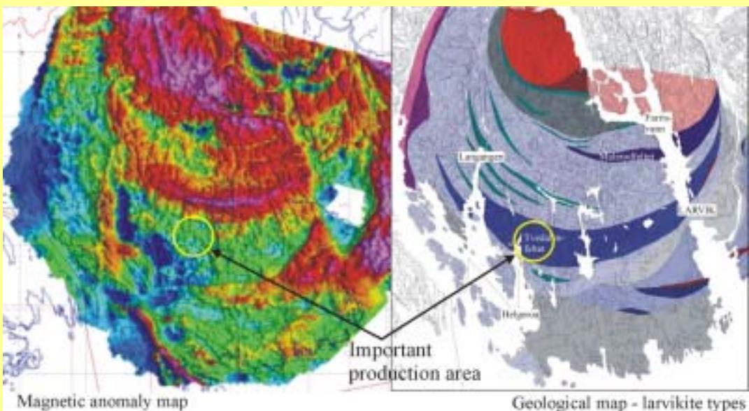
Figure: magnetic anomaly map (left) and geological map of larvikite resources, Southeast Norway. The main quarry area ("Blue Pearl" larvikite) is marked with circles.
