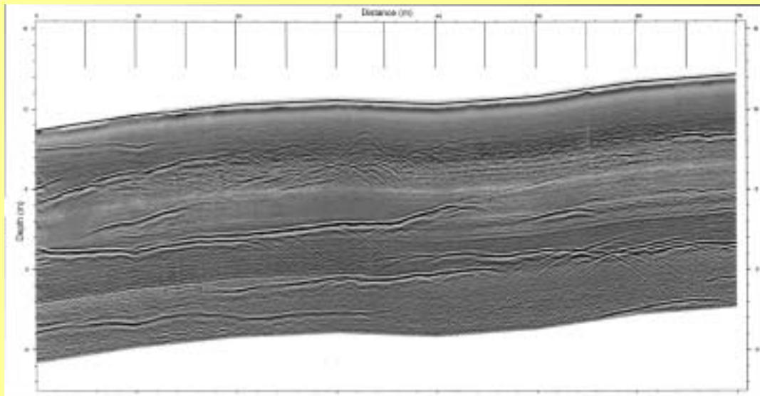
*GPR section from a Finnish granite quarry, showing clearly the horizontal fractures.*
