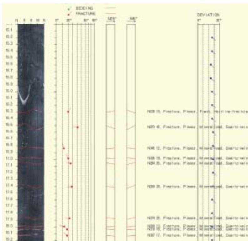
*Optical televiwer* drill hole log. Left - image of drill hole (80 mm in diameter) projected to a flat surface. Interpretation of joint surfaces (directions, groupings and spacing) and layering is done semi-automatically. Source: Geological Survey of Norway (NGU).
