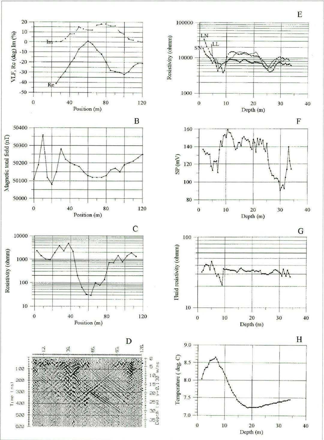
Fig. 2. Surface and borehole geophysics from the Utengen test-site. Left column: VLF (A), magnetics (B), resistivity (C), GPR (D). Right column: formation resistivity (E), SP (F), fluid resistivity (G), temperature (H).
