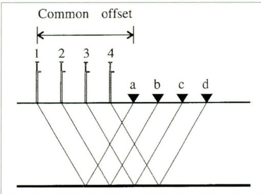
Fig. 4. Common offset profiling.
