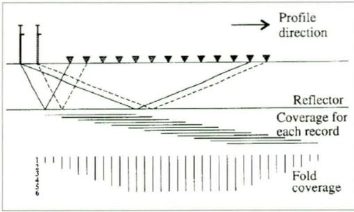
Fig. 2. Common depth point profiling.
