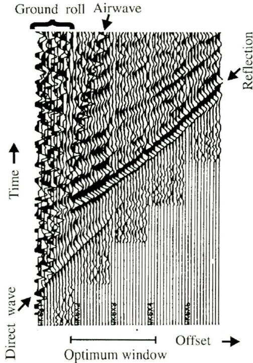
Fig. 1. Common events on a walkaway noise test record.
