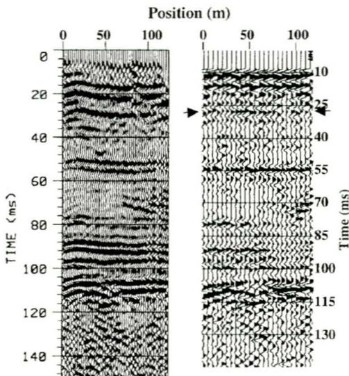
Fig. 6. CDP (left) and CO records derived from the same multi-channel records. Arrows denote shallow, overburden reflector.
