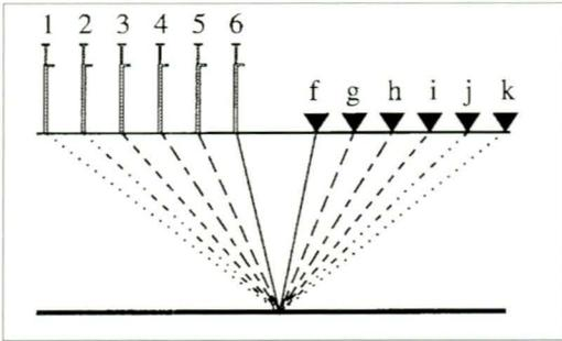
Fig. 3. Example of source-receiver configurations in a CDP gather.
