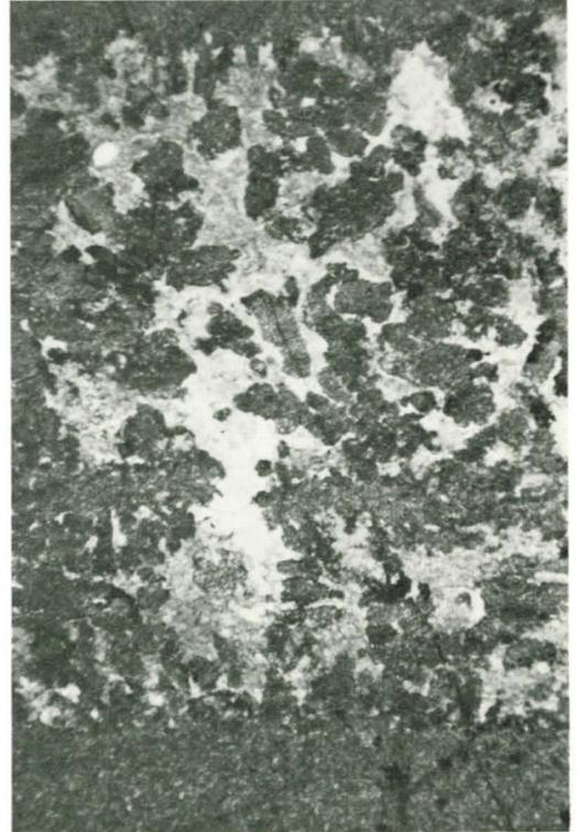
Fig. 6. Random two-pyroxene-plagioclase microstructure in layered hornfels of the Skartasvaggi Formation. In the central parts of the photograph, dark grey: porphyroblasts of pyroxenes (0.5mm). White: quartz and small labradorite grains, medium grey: yellow biotite. Dark grey bands at top and bottom: mainly fine grained pyroxene. Plane-polarised light. Locality: 2550 4750.
