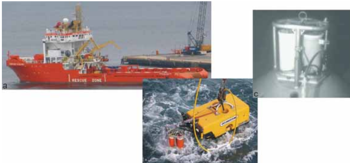
Figure 7.28 Images from the 2002 and 2005 gravimetric surveys at Sleipner. a) Survey vessel. b) ROV with gravimeter (red). c) Gravimeter located on concrete benchmark at seabed.
