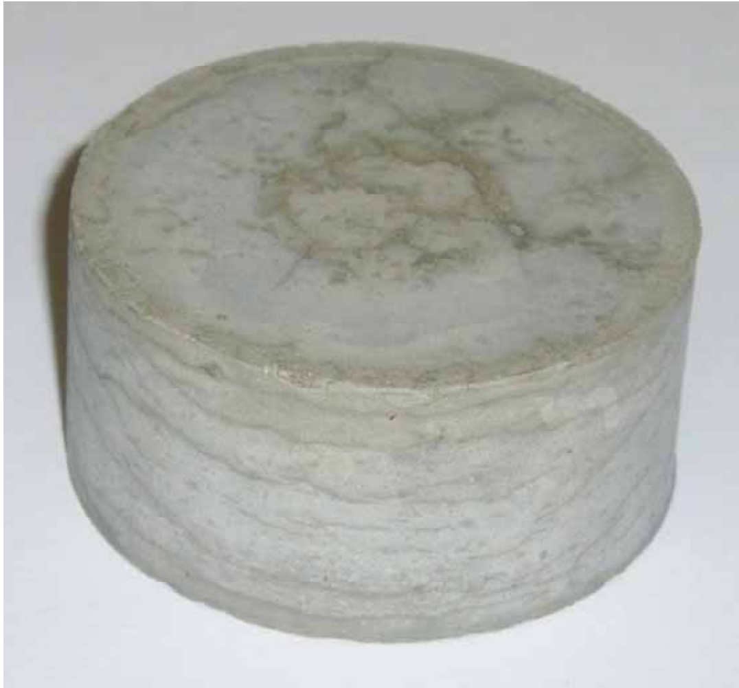
Figure 4.17 Photograph of the Utsira caprock core
