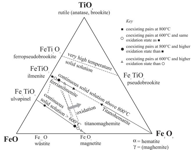
Fig. 3. Composition of oxide minerals in the system  $FeO - Fe_2O_3 - TiO_2$ . The dashed lines between ilmenite and magnetite indicate common geological coexistence at relatively low temperatures, in which magnetite commonly contains ilmenite lamellae. Such intergrowths are formed by the oxidation of magnetite - ulvöspinel followed by oxidation-exsolution of ilmenite. Source could not be located.
