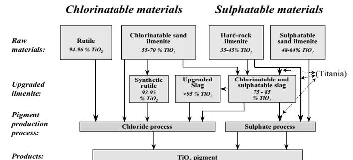
Fig. 4. Paths from titanium raw materials to products (modified from Dormann 1993).
