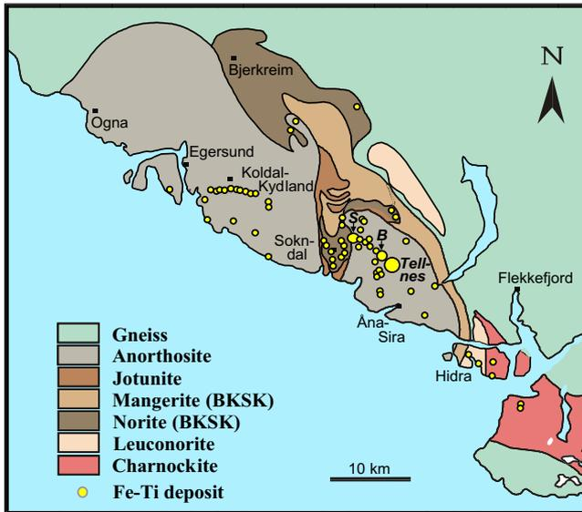
Fig. 2. Simplified geological map and ilmenite ore bodies in the Rogaland anorthosite province. S = Storgangen ilmenite deposit, B = Blåfjell ilmenite deposit. BKSK = rock units belonging to the Bjerkreim-Sokndal intrusion.
