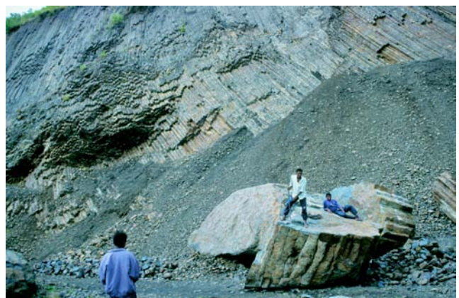
Fig. 15. Quarry in columnar basalt near the town of Ambo.
