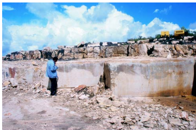
Fig. 9. Sawn limestone bed in a quarry within the Hakimgara limestone deposit, Harar. Note reduction fields in the upper part of the bed.
