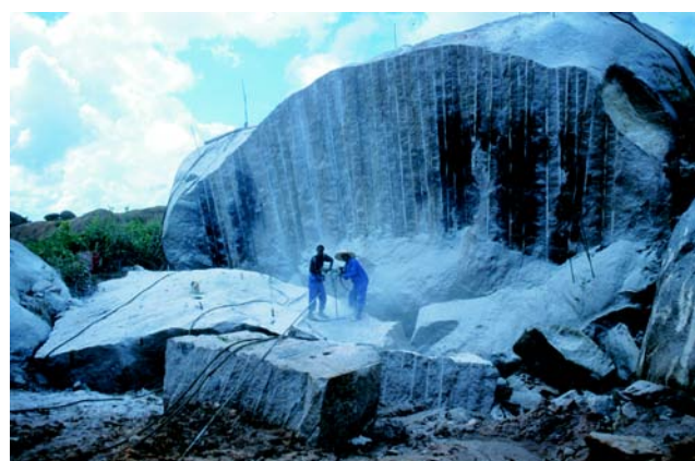
Fig. 5. Quarrying of a giant boulder in the Babile granite deposit, Harar.
