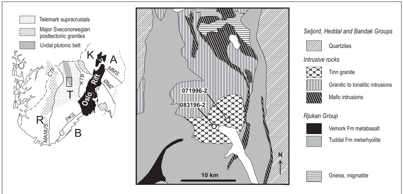
Fig. 1. Simplified geologic map of the Tinn granite and surrounding rocks, compiled from Dons & Jorde (1978) and Sigmond (1998). Overview map: Simplified map of South Norway showing regional subdivision used in this study: A: Østfold-Akershus sector; K: Kongsberg sector; T: Telemark sector; B: Bamble sector; R: Rogaland-Vest Agder sector. Major shear zones: MMS: Mjøsa-Magnor shear zone, ØMZ: Ørje mylonite zone; PKS: Porsgrunn-Kristiansand shear zone; KTB: Kongsberg-Telemark boundary; MANUS: Mandal-Ustaaset line; CTF (broken line): Caledonian thrust front.
